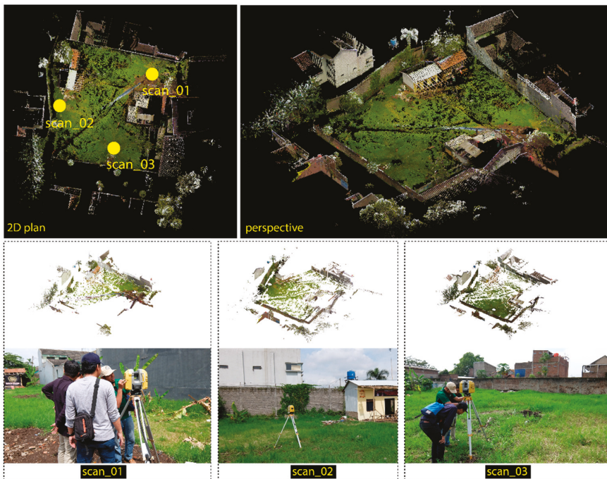
Figure 7. Dataset collection with different views captured in relation to the scanner position.
