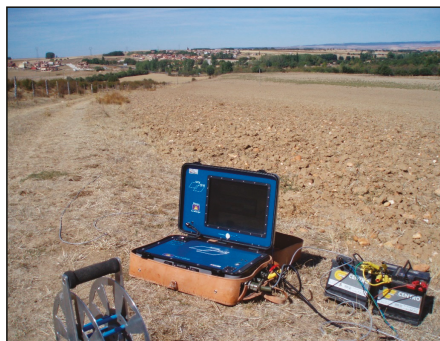
Figure 4. TDEM equipment in the area under study.
