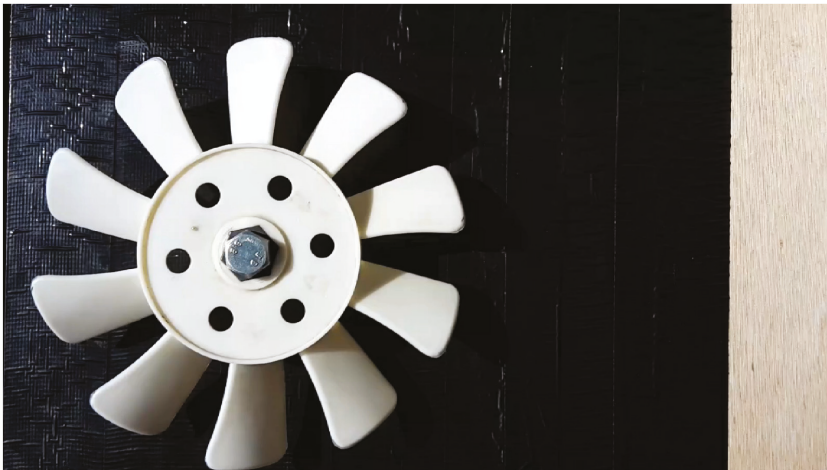
Figure 1. The first frame of the video, digitalized as a 1080 \times 1920 \times 3 matrix: full-HD resolution of 1920 \times 1080 (16:9 aspect ratio), where each pixel color is represented as a triplet of intensities for the three-color components namely red, green, and blue (RGB additive trichromacy color model).
