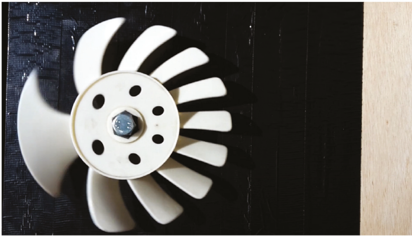
Figure 2. The thousandth frame of the video. The rolling shutter effect is highlighted as a deformation of the blades.
