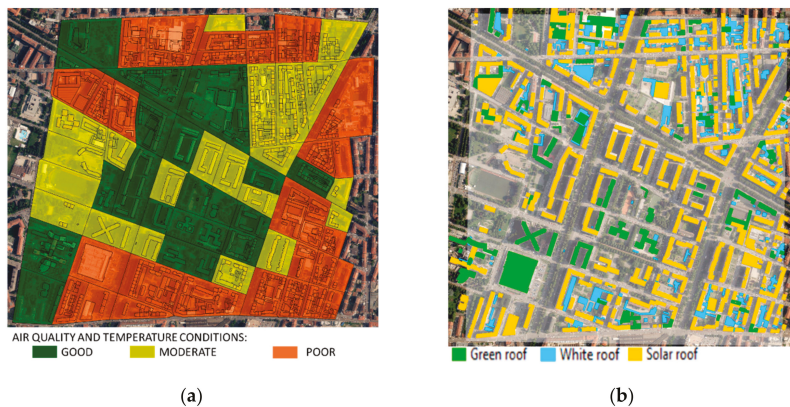
Figure 6. District of Turin with a dimension of 1 km 2 : (a) Building block classification according to three classes of air quality conditions (green, good; yellow, acceptable, red, bad) [23]; (b) analysis of roof potential and feasibility of smart solutions: Green, high-reflectance, and solar roofs.
