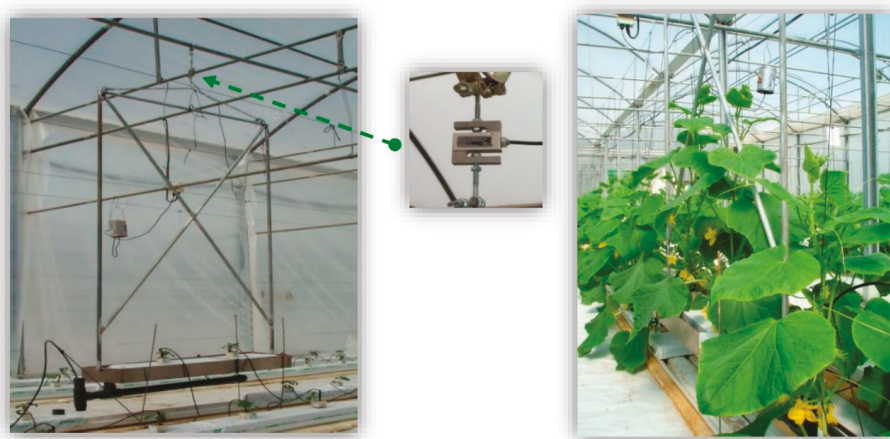
Figure 3. Mounting a lysimeter in a greenhouse structure (left), weighing device S-Beam load cell (centered) and plants grown in a lysimeter (right).
