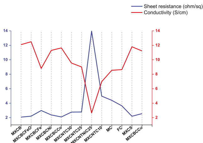
Figure 6. Electric conductivities and sheet resistances of the composites.
