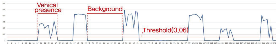
Figure 3. Signal profile from the autoencoder for the test data.
