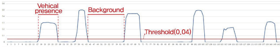
Figure 6. Updated signal profile from the autoencoder when using synthesized images for the test data.
