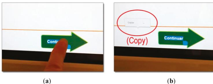
**Figure 1.** Troubles found due to very long pulsations. (a) Text label button selected due to very long pulsation. (b) Secondary button activated (copy) instead clicking on the main action button (the green arrow).
