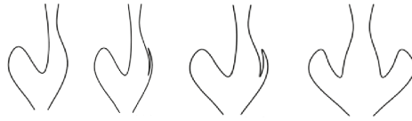
Figure 3. These four images are generated from the same pair of 3D mirror symmetric curves but seen from different vantage points. On the far left, the viewing angle is such that the curve images do not suggest 3D symmetry. Nonetheless, the relationship is there, and it becomes clear as the view is rotated, especially in the two right-most images. These images were published in [28].
