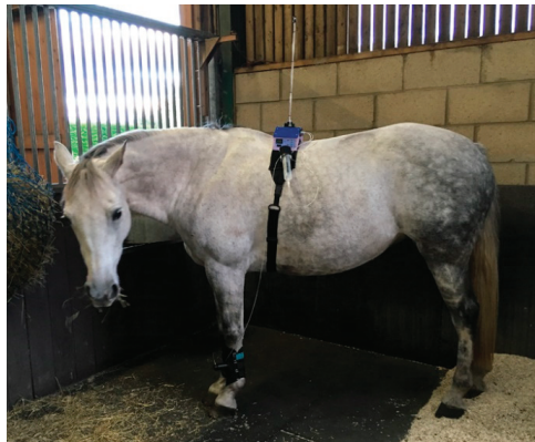
Figure 8. Horse with mechanical system in place: control unit and reservoir mounted on the back, with pressure line to the actuator on the foreleg.
