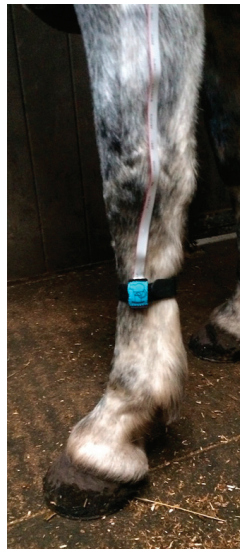
Figure 6. Thermal probe positioned on the limb with a carefully tensioned elastic and Velcro® band.
