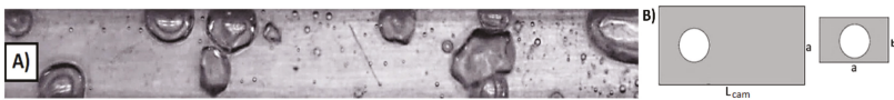
Figure 5. (A) Actual and (B) approximated shapes of vapor bubbles in longitudinal and transverse sections of the channel with flow direction, case I. Water, T_{in} = 63.1\text{ }^{\circ}\text{C} , T_{out} = 123.8\text{ }^{\circ}\text{C} , p_{in} = 1.165\text{ bar} , \Delta p = 0.0024\text{ bar} , q = 298.7\text{ kW/m}^2 , G = 7.2\text{ kg/(m}^2\text{ s)} , Re = 55.0 , L_{cam} = 20\text{ mm} .
