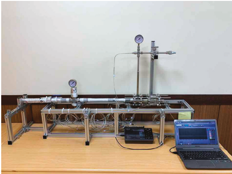
Figure 4. Photograph of the experimental apparatus for the vortex tube.
