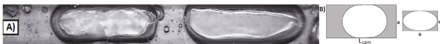
Figure 6. (A) Actual and (B) approximated shapes of vapor bubbles in longitudinal and transverse sections of the channel with flow direction, case II. Water, T_{in} = 55.2\text{ }^{\circ}\text{C} , T_{out} = 125.9\text{ }^{\circ}\text{C} , p_{in} = 1.0697\text{ bar} , \Delta p = 0.0016\text{ bar} , q = 260.1\text{ kW/m}^2 , G = 8.6\text{ kg/(m}^2\text{ s)} , Re = 66.9 , L_{cam} = 20\text{ mm}
