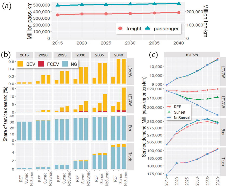
Figure 5. Service demand in the road transportation sector. Note: Total service demand: (a), Technology share (b), Service demand of ICEVs (c). The rest of the percentage of bars in (b) is the share of service demand for refined liquid vehicles.
