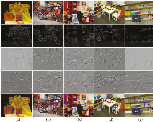
Figure 4. The similarity cost functions and the shape of the adaptive support window. (a) Jade plant; (b) motorcycle; (c) playroom; (d) play table; and (e) shelves. From top to bottom: the reference images; the modulus images of the illumination normal vector; the gradient maps along horizontal direction; the gradient maps along vertical direction; and the examples of the adaptive support window.
