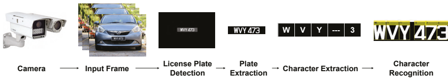
Figure 1. Outline of the proposed system for automatic license plate recognition.
