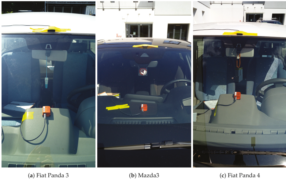
Figure 1. Placement of the sensor used for the data collection in the vehicles for three vehicle models.
