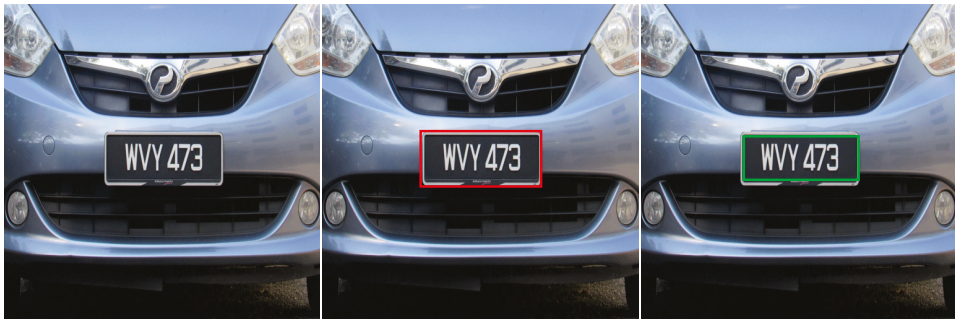
Figure 4. Detection result: from left to right, input image, ground truth image (red bounding box), and output image with detected license plate ROI (green bounding box).
