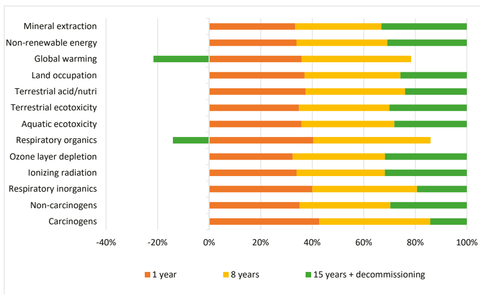
Figure 4. Life-cycle assessment of a 500-kW heat output Stirling cycle-based HP.
