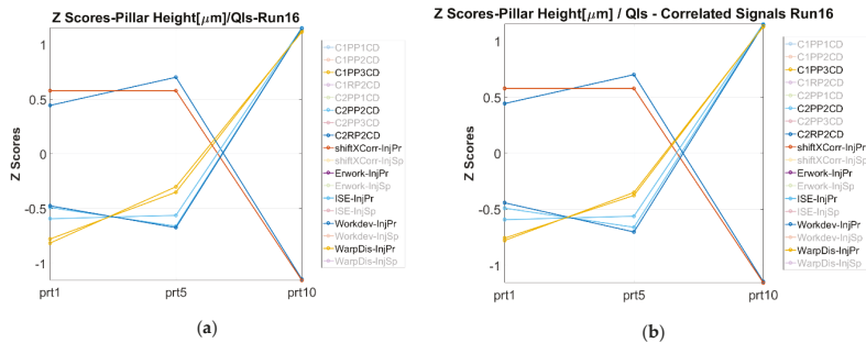
Figure 16. Example of process fingerprint candidates to measurand trends for experimental run 16 based on (a) nominal signals and (b) cross correlated signals. The legend of the graphs denotes both the measurand datasets (i.e., C1PP1: Cavity 1–Position PP1) and the deviation based (Type 1) “process fingerprints”.
