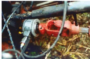
**Figure 3.** Required torque and power sensor arranged at the tractor power take-off (PTO).
