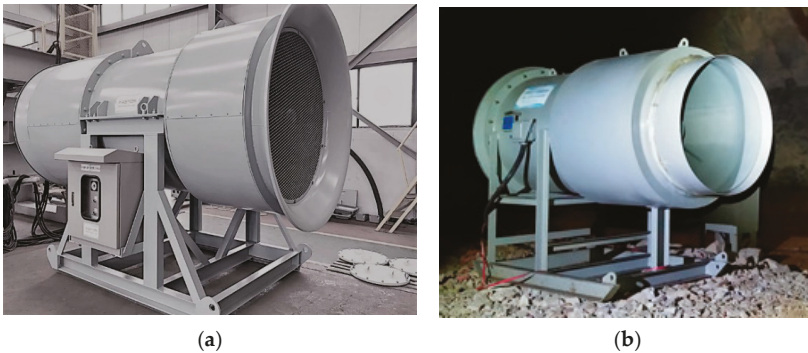
Figure 2. Two fans developed for the pressurization ventilation experiments: (a) 37 kW high-pressure fan; (b) 15 kW low-pressure fan.
