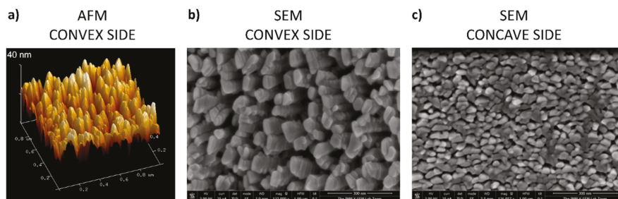
Figure 5. Microscopy images of the DePuy Synthes plate after deposition of Ti nanocolumns: (a) Atomic force microscopy (AFM) topographic map of the convex side of the plate; (b) SEM image of the nanocolumnar structures in the convex and (c) concave side of the plate.
