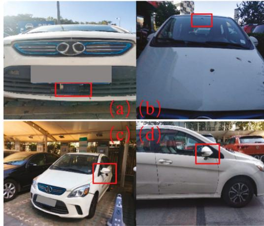
**Figure 1.** Data acquisition equipment mounted on the vehicle. Figure (a) shows the millimeter wave radar. Figures (b–d) show the cameras.
