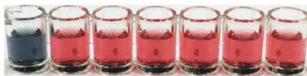
Figure 17. Selectivity of aptamer-modified gold nanoparticles for streptomycin. From left to right: streptomycin, amoxicillin, tetracycline, oxytetracycline, carbamazepine, diclofenac and penicillin added to aptamer-modified gold nanoparticles, ABTS and H 2 O 2 . (Reprinted with permission from [164]. Copyright © The Authors. Distributed under a Creative Commons (CC BY-NC) license).
