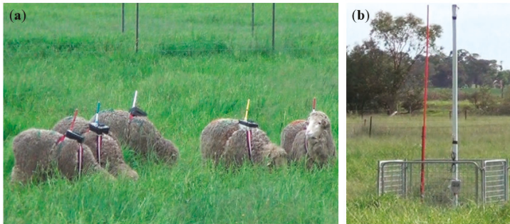
Figure 4. RTK rovers fitted on the back of sheep via harnesses (a), and fixed base station (b) in the middle of the paddock. The two masts (b) were for the GNSS amplified antenna, and RTK correction transmitter.
