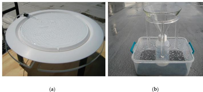
**Figure 2.** (a): Dry deposition sampler. Plate diameter is 35 cm. (b): Wet deposition sampler. Funnel diameter is 20 cm.
