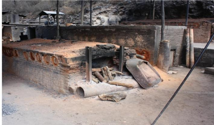
**Figure 3.** Wood-fired ovens at an artisanal primary mercury mine in Camargo, Peñamiller Municipality, State of Querétaro Arteaga, Mexico. Photo taken in February 2017 by Bruce Marshall.
