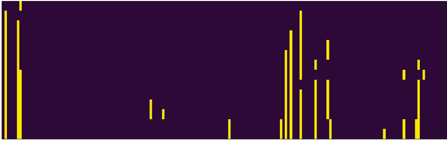
Figure 12. Visualization of optimal features for different feature subset sizes. The x axis represents the feature index, while the y axis depicts the number of features k (increasing with each row). FASTENER does not simply add new features as k is increased, but rather finds the best possible combination of features that gives the best possible classification result for a given k .
