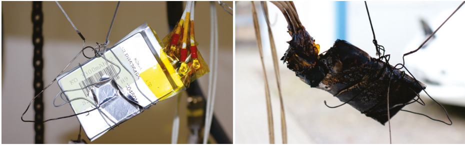
Figure 7. Experiment HT1: Left: Cell with applied temperature sensors before the experiment. Right: Cell after the experiment.
