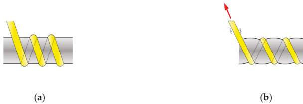
Figure 2. Schematic depicting the manufacturing of glass fiber-reinforced polymer (GFRP) reinforcing bars (rebars). (a) general braiding. (b) modified braiding.
