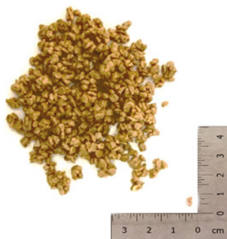
Figure 2. Form-stable LS/PEG composite obtained through the vacuum impregnation process.
