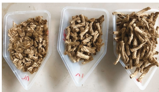
Figure 2. The physical appearance of the jute fibers used in this study, which were cut into different length.
