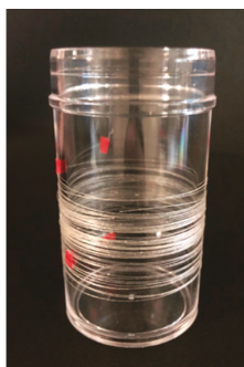
Figure 3. Photograph of the chitosan–TMSA microfiber (ChTMSA001).
