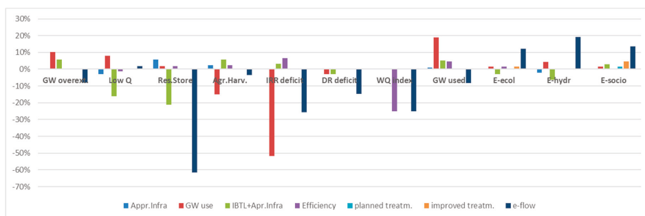
Figure 10. Percent change in basin-wide indicator values for intervention strategies. Values relative to the business as usual scenario. Increases indicate improvement and reduction indicate deterioration.
