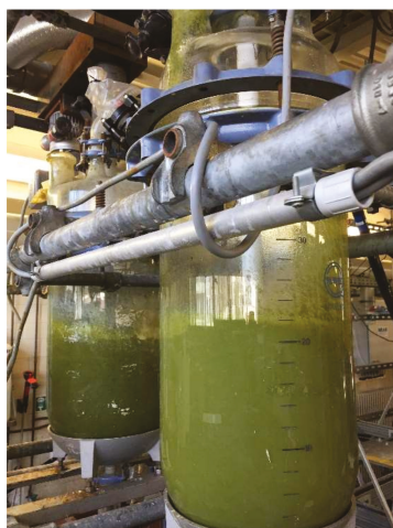
Figure 14. Treatment of eudialyte concentrate in two reactors at the Institute of Process Metallurgy and Metal Recycling (IME) demonstration plant, RWTH Aachen.
