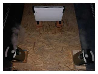
Figure 6. Box indoor hygrothermal control equipment.
