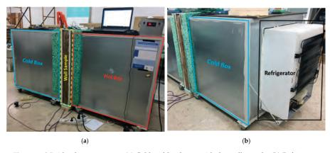
Figure 8. Mini hot box apparatus: (a) Cold and hot boxes with the wall sample; (b) Refrigerator attached to the cold box.
