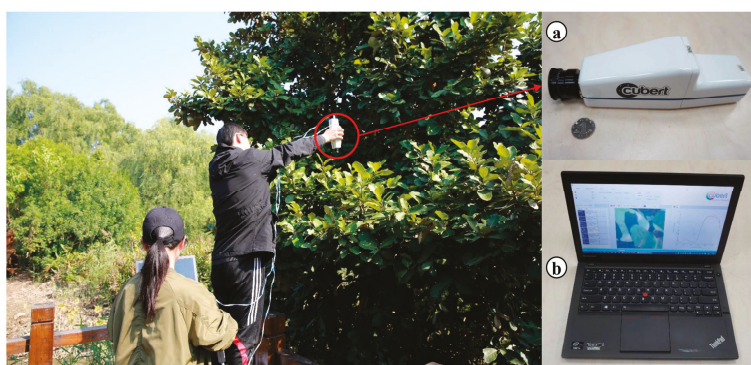
Figure 3. Field hyperspectral measurements above the mangrove canopies and the set-up used to acquire the hyperspectral images. (a) The UHD 185 hyperspectral imaging sensor, and (b) a notebook computer.
