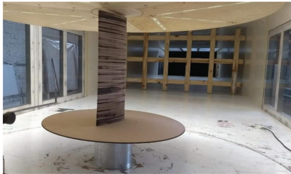
Figure 5. Airfoil model mounted inside the FLOW wind tunnel, with the turbulence grid installed in the background.
