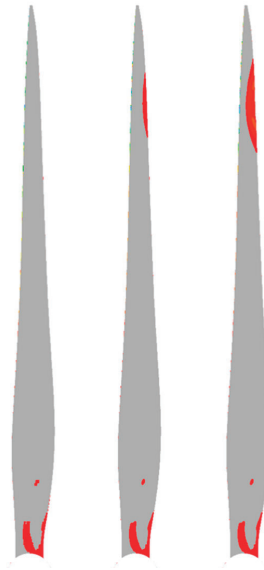
Figure 9. Zero net flow rate gusts separation region (in red) over the blade suction side at 90^\circ azimuth angle: (left) unguasted case, (center) case with A_g = 5 m/s, and (right) case with A_g = 10 m/s.
