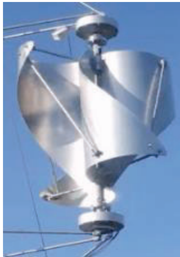
Figure 2. RW IceWind turbine.
