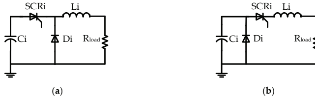
Figure 3. Two simplified PFU topologies. (a) Simplified type I PFU topology; (b) simplified type II PFU topology.
