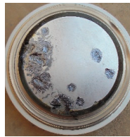
Figure 16. Photograph of the damaged thyristor.
