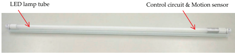
Figure 2. LED sensor energy-saving lamp (T5 mountain ceiling lamp).
