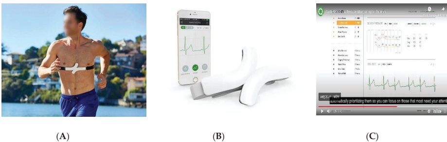
Figure 4. QardioMD ECG solution (QARDIO MD system). (A) QardioCore ECG—chest strap with electrode. (B) Qardio mobile app (ECG recording on iPhone) and chest strap (QardioCore ECG) with electrode. (C) ECG recording on QardioMD remote monitoring web-based portal.
