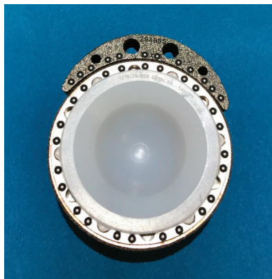
Figure 1. Photograph of acetabular cup, augment and liner. Note the attached optical marker points along the rim of the cup and augment.
