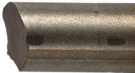
Figure 9. Magnified lateral view of Ti-CG post biomechanical testing: fatigue fracture of the rod at the rod-screw junction, illustrating surface marks of the tightened screws on the rod.
