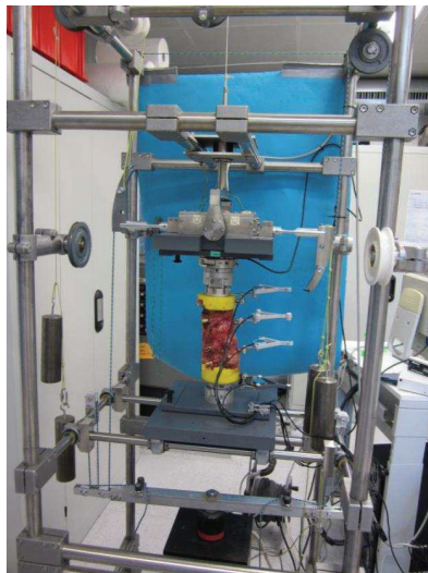
Figure 2. Spine tester (Schunk FT Delta SI 660-60, Lauffen/Neckar, Germany) with six degrees of freedom; three in translation (green) and three in rotation (orange). Specimen embedded in PMMA.
