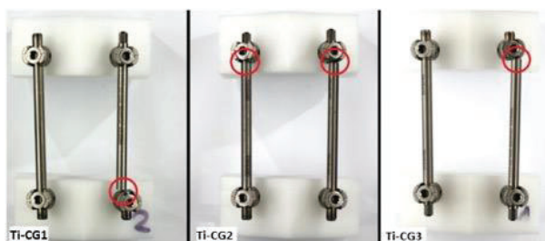
Figure 3. Sites of rod fracture of titanium control group (Ti-CG) post biomechanical testing and fatigue fractures of the rods at the rod-screw junction.
