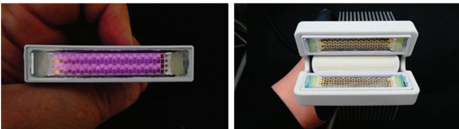
**Figure 7.** Photograph of an LED array developed by CYBERDYNE INC with four rows of LED elements, in which Rows 1 and 3 are 850 nm elements, and Rows 2 and 4 are 750 nm elements (left). In this picture, the 850 nm elements are activated and captured using an IR camera. Photograph of a LED-based PA/US probe developed by CYBERDYNE INC, in which two LED arrays (750/850 nm) are placed on both sides of a linear array US probe (7 MHz) (right).
