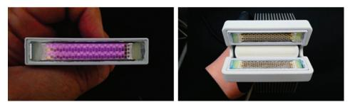
**Figure 7.** Photograph of an LED array developed by CYBERDYNE INC with four rows of LED elements, in which Rows 1 and 3 are 850 nm elements, and Rows 2 and 4 are 750 nm elements (**left**). In this picture, the 850 nm elements are activated and captured using an IR camera. Photograph of a LED-based PA/US probe developed by CYBERDYNE INC, in which two LED arrays (750/850 nm) are placed on both sides of a linear array US probe (7 MHz) (**right**).
