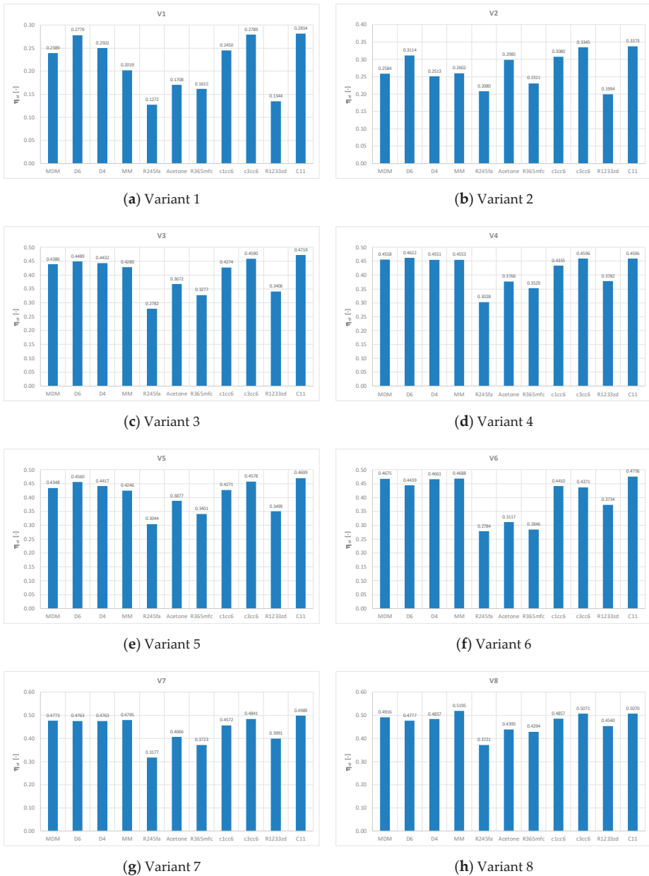
Figure 8. Overall efficiency for different working media: (a) Variant 1; (b) Variant 2; (c) Variant 3; (d) Variant 4; (e) Variant 5; (f) Variant 6; (g) Variant 7; (h) Variant 8.
