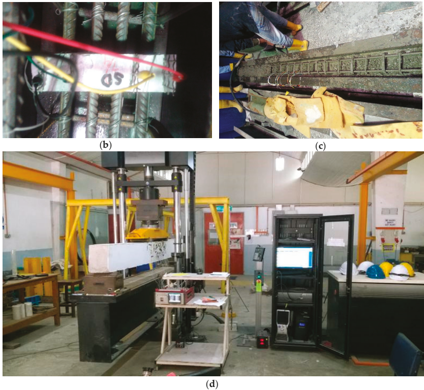
Figure 1. Description of specimen and test setup (a) Dimensions of graphene–cement composite specimen with wire mesh details; (b) placement of specimen on reinforcement; (c) casting of reinforced concrete (RC) beam; and (d) overall test setup for measuring the electrical properties of graphene–cement composite specimen in the RC beam.
