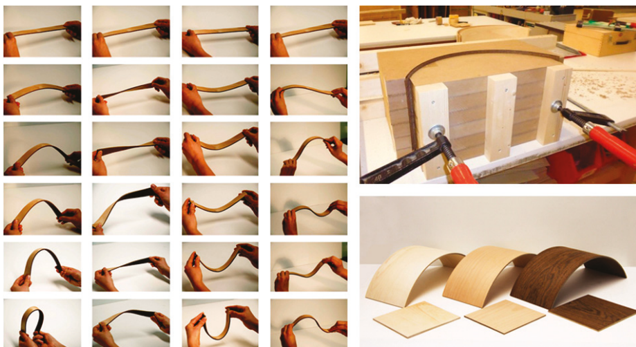
Figure 3. Illustration of the flexibility of the Bio-flexi panel when veneered from one side and how it can be veneered from both sides to fix the geometry intentionally (republished: [91]).
