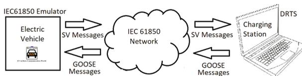
**Figure 22.** HIL test set-up for model validation.
