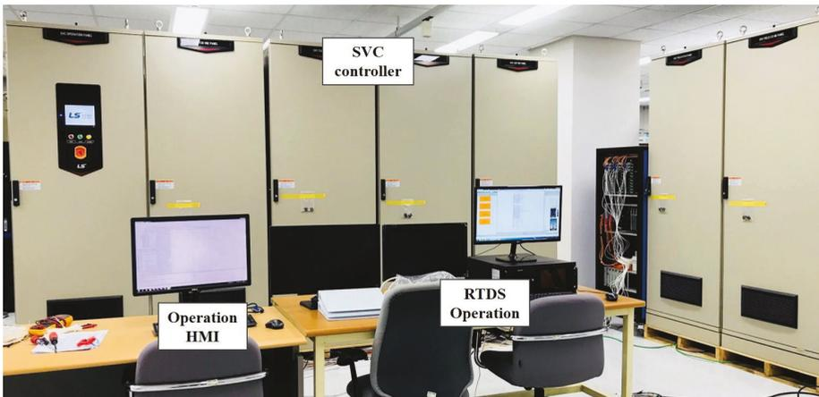
Figure 8. SVC controller interfaced with RTDS.
