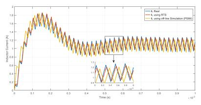
Figure 14. Inductor current of the real buck converter: real-time simulation and PSIM.
