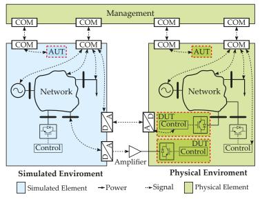
Figure 2. Generic scheme describing the Power System Hardware-in-the-Loop (PSHIL) configuration.
