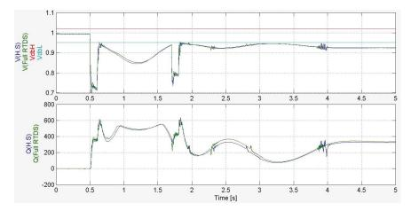
**Figure 13.** A 765 kV line fault is applied nearby Shin-Jecheon; Shin-Jecheon bus voltage (first row) and reactive power of SVC (second row); RTHS (blue line) and large-scale RTS (green line).
