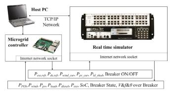
Figure 14. Rule based microgrid controller design and validation testbed [37].
