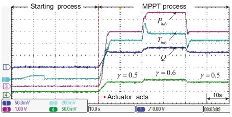
**Figure 14.** Hydraulic dynamics process in the real-time simulation,  $P_{hdy}$  the generated hydraulic power (100 w/div),  $T_{hdy}$  the turbine torque (2 N·m/div), Q the water flow rate (0.05 m<sup>3</sup>/s/div).
