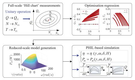
Figure 1. Procedure of a 'Hill Charts' based modelling.
