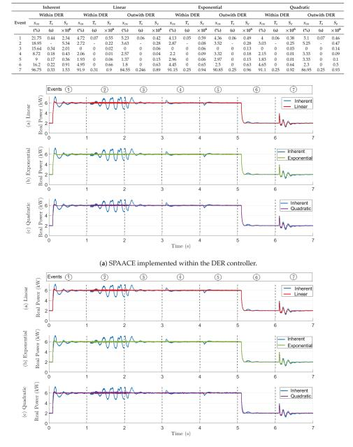
Table 4. Dynamic response performance indicators for the seven events under the grid-connected mode for operation.
