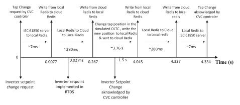
Figure 16. Time delays introduced in the setup.
