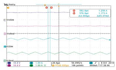
**Figure 18.** Output signals of the real converter and HIL simulation with a time delay, simulated voltage (Channel 1), simulated current (Channel 2), real voltage (Channel 3), and real current (Channel 4).
