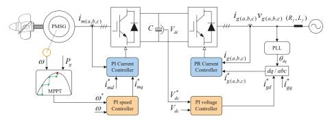
Figure 11. Control design diagram of grid-connected VS-HEP.
