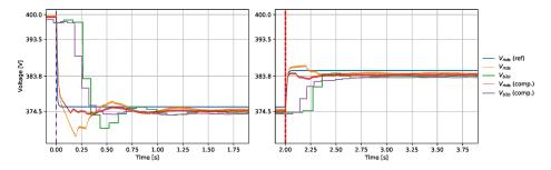
Figure 12. Inset graphs of voltage response during closed-loop test: DL step (left); and OLTC tap change (right).
