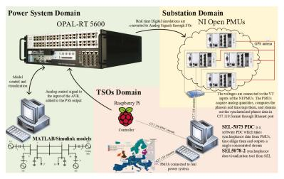
Figure 7. Controller Hardware-in-the-Loop (CHIL) testbed setup for controller validation.
