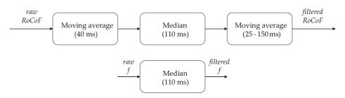
Figure 7. The configuration of filtering applied to the reported frequency f and RoCoF.
