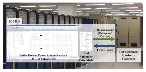
Figure 1. Configuration of dynamic performance test (DPT) for equipment.
