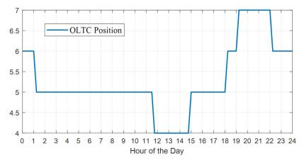
Figure 15. On Load Tap Changer (OLTC) position changes.
