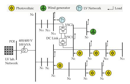
Figure 5. One-line diagram of the MV physical network within the PSHIL infrastructure at the University of Sevilla.
