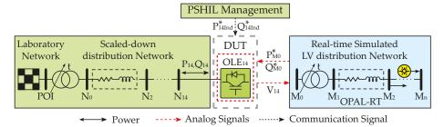
**Figure 8.** PSHIL application example. Integration of the LV real-time simulated network and the physical MV network.
