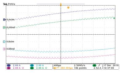
**Figure 20.** Zoomed output currents ( $i_a$  and  $i_b$ ) of the three-phase VSI and HIL simulation, simulated  $i_a$  current (Channel 1), simulated  $i_b$  current (Channel 2), real  $i_b$  current (Channel 3), and  $i_a$  real current (Channel 4).
