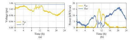
Figure 14. PSHIL-3. (a) 24-h evolution of voltage in bus M7. (b) 24-h evolution of PV active and reactive power injections in bus M7.
