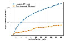
Figure 16. Parallelization results for eight threads comparing different decoupling methods.
