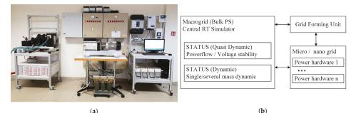
Figure 1. Power Hardware-in-the-Loop (PHIL) TU-Sofia Power System Stability Laboratory. (a) Micro/ nanogrid lab setup; (b) Lab architecture.
