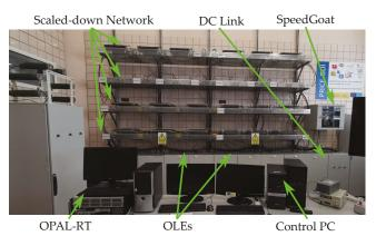
Figure 4. PSHIL layout of the Department of Electrical Engineering at the University of Sevilla.
