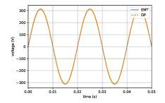
**Figure 12.** Capacitor voltage of a DP inverter model including the fundamental and eight harmonics compared to a Simulink EMT model.
