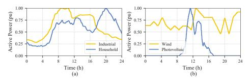
Figure 9. PSHIL application example. Daily profiles in per-unit (a) Load profiles, (b) Generation profiles.
