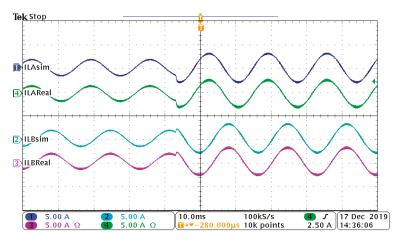
**Figure 19.** Output currents ( $i_a$  and  $i_b$ ) of the three-phase VSI and HIL simulation, simulated  $i_a$  current (Channel 1), simulated  $i_b$  current (Channel 2), real  $i_b$  current (Channel 3), and  $i_a$  real current (Channel 4).
