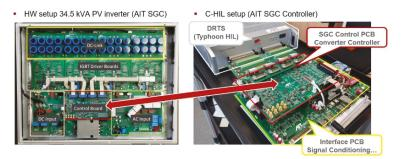
Figure 19. CHIL islanding testbed with AIT SGC HIL controller connected to Typhoon-HIL RTSM.
