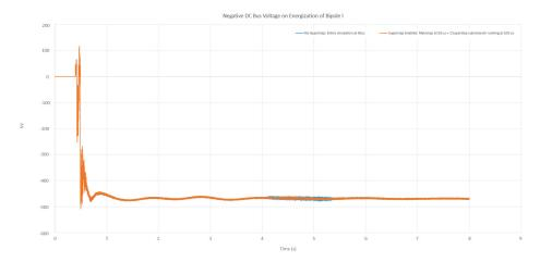
**Figure 2.** Simulation results showing negative DC bus voltage of an HVDC bipole upon energization for a single-rate simulation at 50 µs (blue curve) vs. a multi-rate simulation including a Superstep subnetwork running at 100 µs (orange curve).
