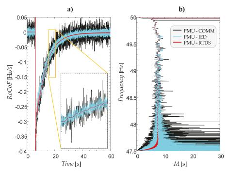
**Figure 3.** The *RoCoF(t)* report of three applied sources (PMU-IED, PMU-COMM and PMU-RTDS) after an RTDS simulation of an active power deficit (**a**) and a corresponding frequency versus frequency stability margin diagram (**b**).
