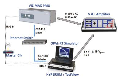
Figure 26. HIL testbed for pre-certification of a phasor measurement unit (PMU).
