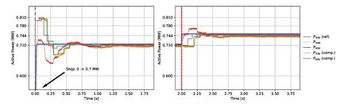
Figure 13. Inset graphs of power change during: DL step (left); and OLTC tap change (right).
