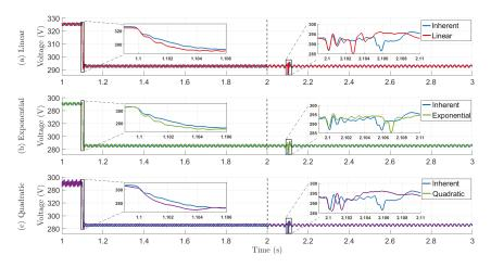
Figure 7. Dynamic response evaluation of SPAACE under the islanded mode of operation. SPAACE is implemented outwith the DER controller.
