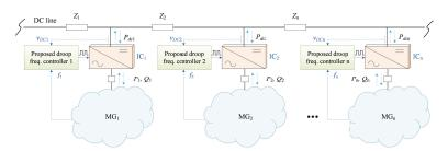
**Figure 10.** Proposed stand-alone multi-microgrid system [43]. Reproduced with permission from Hyeong-Jun Yoo, A Droop Frequency Control for Maintaining Different Frequency Qualities in a Stand-Alone Multimicrogrid System; published by IEEE, 2018.
