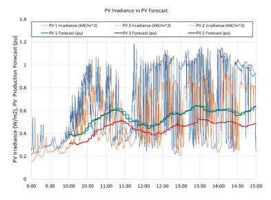
Figure 10. Irradiance and PV Energy Forecast Profiles. 1000 W/m<sup>2</sup> produces 1pu of Active Power.
