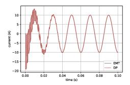
Figure 4. Comparison of DP and electromagnetic-transient (EMT) resistor current results for the transmission line model.
