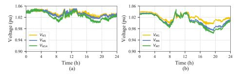
**Figure 13.** PSHIL-2. Impact on the MV and LV distribution networks. (a) 24-h evolution of the MV network voltages at buses N3, N6, and N14. (b) 24-h evolution of the LV network voltages at buses M1, M4, and M7.
