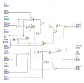
Figure 5. Discrete buck converter model programming in LabVIEW.
