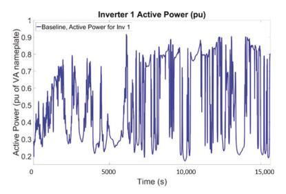
Figure 6. PV power levels for 4- hour simulation.
