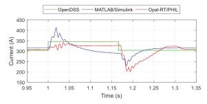
**Figure 6.** Comparison between physical photovoltaic (PV) inverter currents during a 3Ø Fault at Bus 4 [25]. Reproduced with permission from Rachid Darbali-Zamora, Feeder Fault Comparison Utilizing a Real-Time Power Hardware-in-the-Loop Approach for Photovoltaic System Applications; published by IEEE, 2019.
