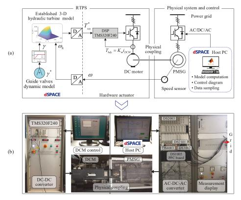
**Figure 10.** PHIL-based hybrid real-time VS-HEP simulation system, (a) global design diagram, with  $T_{hdy}$  the emulated hydraulic torque,  $K_m$  the torque constant,  $i_{DCM}$  the direct current of DCM, (b) PHIL experiment benchmark
