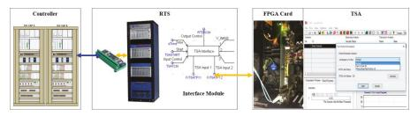
Figure 4. Configuration of real-time hybrid simulator (RTHS).
