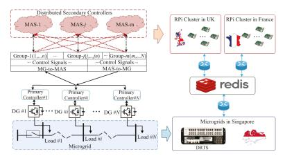
**Figure 23.** Geographically distributed CHIL for advanced validation of a distributed control algorithm [72]. Reproduced with permission from Efren Guillo-Sansano, A Distributed Control Scheme of Microgrids in Energy Internet and Its Multi-Site Implementation; published by IEEE, 2020.
