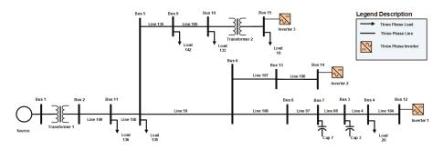
Figure 3. One Line Diagram of PNM Feeder.
