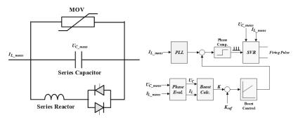
Figure 4. Thyristor Controlled Series Compensator (TCSC) topology and conceptual control block.
