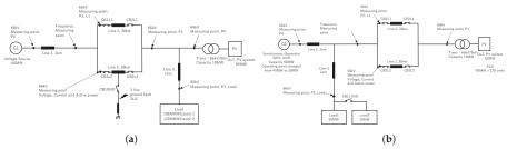
**Figure 18.** Power system for combination test for (**a**) volt-var and low voltage ride through and (**b**) frequency-watt and other functions.
