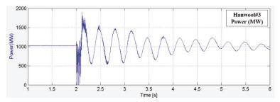
Figure 15. Time domain simulation result in light load of generator.
