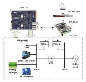
Figure 12. HIL test set-up for model validation.
