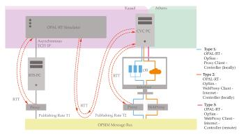
**Figure 24.** Test setup for geographically distributed co-simulation with OpSim [59]. Reproduced with permission from Juan Montoya, Asynchronous Integration of Real-Time Simulators for HIL-based Validation of Smart Grids; published by IEEE, 2019.
