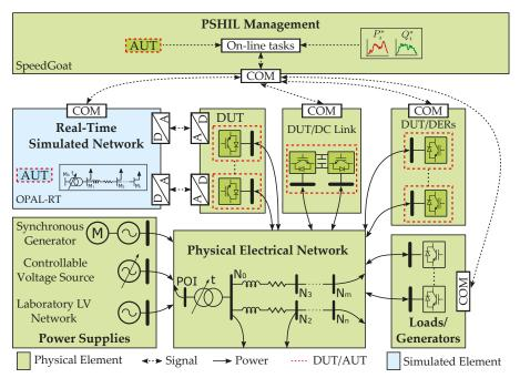
Figure 3. PSHIL platform of the Department of Electrical Engineering at the University of Sevilla.
