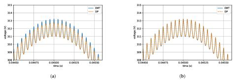
**Figure 13.** Ripple of the capacitor voltage of a DP inverter model including the fundamental and 8 harmonics (**a**) or 28 harmonics (**b**) as compared to a Simulink EMT model.
