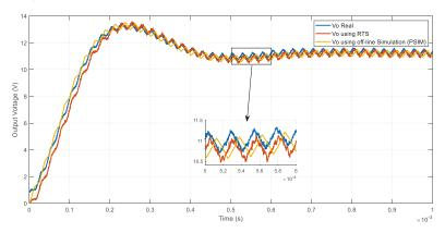
Figure 15. Output voltage of the real buck converter: real-time simulation and PSIM.
