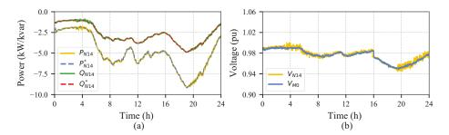
**Figure 10.** PSHIL-1: N14 industrial load and integration of the LV real-time simulated network within the MV scaled-down physical system. (a) 24-h evolution of active and reactive power injected by the OLE connected to bus N14. (b) 24-h evolution of voltages in bus N14 (physical network) and M0 (real-time simulated network).
