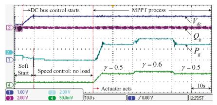
**Figure 16.** Grid-side control performance, the DC-link voltage  $V_{dc}$  (100 V/div), the active power  $P_g$  (200 W/div), the reactive power  $Q_g$  (200 VarA/div).
