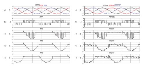
**Figure 3.** Simulation results for a neutral point clamped (NPC) converter modelled with resistive switching based on a predictive algorithm (left) and L/C associated discrete circuits (right): (a) AC side currents, (b) internal phase A voltage, (c) current through phase A upper valve 1, (d) current through phase A upper valve 2, (e) current through phase A lower valve 1.
