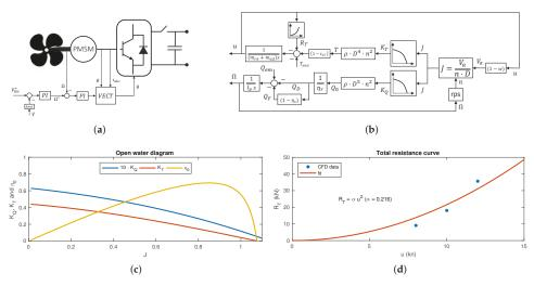
Figure 7. (a) Propulsion system layout; (b) propulsion plant model; (c) propeller open water diagram and (d) ship hull total resistance curve.
