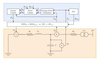
Figure 1. Averaged inverter model with controls.
