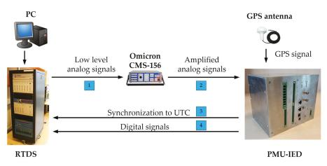
Figure 8. A graphical representation of a real-time digital simulation setup.
