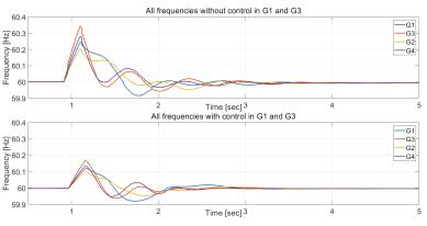
Figure 8. Frequency response without and with controller.
