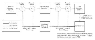
Figure 17. Megawatt scale PHIL setup for smart inverter assessment test.
