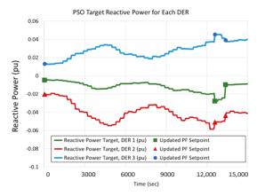
**Figure 12.** PSO PNM target reactive power levels for each distributed energy resources (DER). The target reactive power is calculated from the PSO power factor (PF) set point and the PV forecast at that time.
