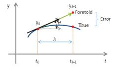
Figure 3. Graphic representation of the general solution using numerical methods.
