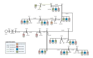
Figure 4. One-line diagram of National Grid (NG) feeder.
