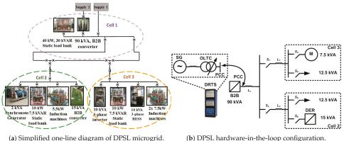
(b) DPSL hardware-in-the-loop configuration.
