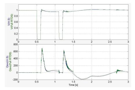
Figure 9. A 345 kV line fault is applied at Shin-Jecheon bus; Shin-Jecheon bus voltage (first row) and reactive power of SVC (second row); RTHS (blue line) and large-scale RTS (green line).
