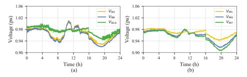
**Figure 11.** PSHIL-1. Impact on the MV and LV distribution networks. (**a**) 24-h evolution of the MV network voltages at buses N3, N6, and N14. (**b**) 24-h evolution of the LV network voltages at buses M1, M4, and M7.
