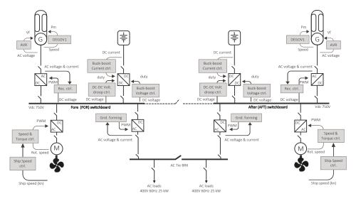
Figure 4. Shipboard microgrid main control loops.
