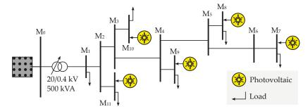
Figure 7. PSHIL application example. One-line diagram of the LV real-time simulated network.
