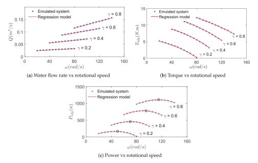
**Figure 12.** Static hydraulic features assessment, (**a**) water flow rate vs rotational speed, (**b**) hydraulic turbine torque vs rotational speed, and (**c**) output hydraulic power vs rotational speed.
