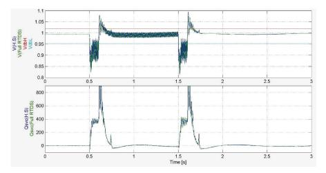
Figure 10. A 345 kV line unbalanced fault is applied at Shin-Jecheon bus; Shin-Jecheon bus voltage (first row) and reactive power of SVC (second row); RTHS (blue line) and large-scale RTS (green line)
