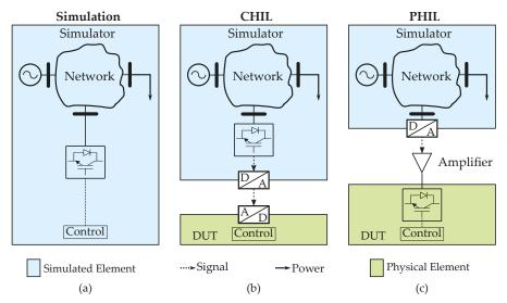
**Figure 1.** Possible testing setups for assessing the effect of a new smart grid technology in the power system: (a) Simulation, (b) Control Hardware-in-the-Loop (CHIL), (c) Power-Hardware-in-the-Loop (PHIL).
