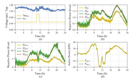
**Figure 12.** PSHIL-2. DUT performance using 24-h evolution of: (**a**) OLTC tap position and voltage of bus N3. (**b**) DER reactive power injections in buses N3 and N6. (**c**) DC-link reactive power injections. (**d**) DC-link active power transfer from N8 to N14.
