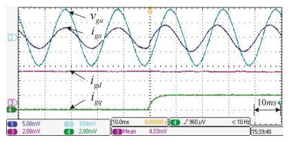
**Figure 17.** Grid-injected current control,  $i_{ga}$  the grid current of phase A (5 A/div),  $v_{ga}$  the grid voltage of phase A (100 V/div),  $i_{ga}$  the reactive current (2 A/div),  $i_{gd}$  the active current (2 A/div).
