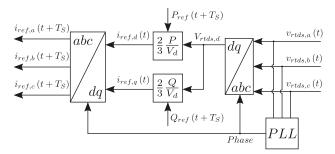
Figure 8. Calculation of the current reference.
