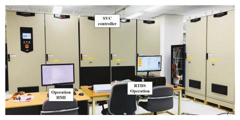
Figure 8. SVC controller interfaced with RTHS.
