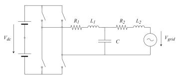
**Figure 11.** Single phase inverter with LCL output filter connected to an equivalent grid represented by a voltage source with series impedance  $R_g$  and  $L_g$ .
