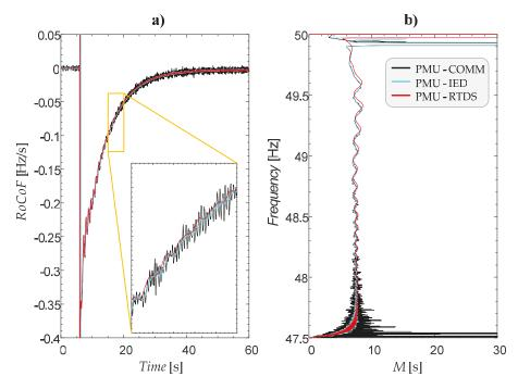
**Figure 4.** The improvement in reported *RoCoF(t)* after applying a moving average filter to the PMU-IED and the PMU-COMM (**a**), and a corresponding frequency versus frequency stability margin diagram (**b**).
