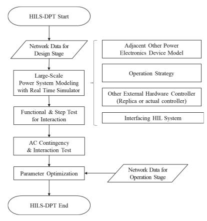
**Figure 2.** The entire procedure of hardware-in-the-loop simulation for dynamic performance test (HILS-DPT) using a large-scale real-time simulator (RTS).
