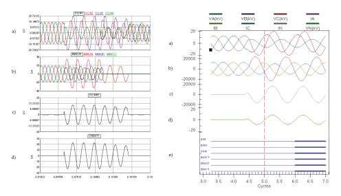
**Figure 6.** Results for testing a commercial relay for a stator-ground generator fault at 50% from the neutral. Simulation results (**left**): (**a**) stator voltages, (**b**) stator currents, (**c**) neutral voltage, (**d**) neutral current; relay recorded events (**right**): (**a**) stator voltages, (**b**) stator currents, (**c**) neutral current, (**d**) neutral voltage, (**e**) digital signals.
