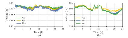
Figure 15. PSHIL-3. Impact on the MV and LV distribution networks. (a) 24-h evolution of the MV system voltage in buses N3, N6, and N14. (b) 24-h evolution of the LV system voltage in buses M1, M4, and M7.
