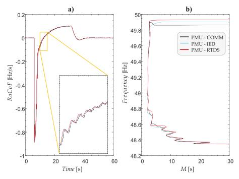
**Figure 6.** The improvement in reported *RoCoF* dynamics after applying a median filter to the PMU-IED and the PMU-COMM (**a**), a corresponding frequency versus frequency stability margin diagram (**b**).
