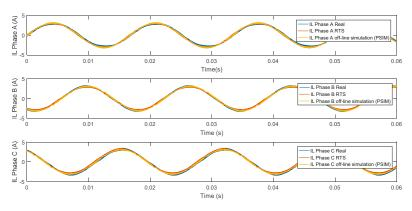
Figure 16. Phase current of the three-phase VSI, real-time simulation and PSIM.
