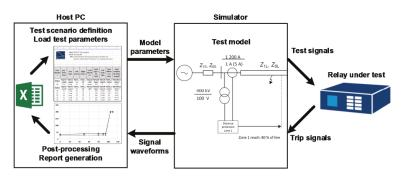
Figure 5. Workflow of the distance protection relay testing.
