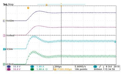
**Figure 17.** Output signals of the real converter and HIL simulation, simulated voltage (Channel 1), simulated current (Channel 2), real voltage (Channel 3), and real current (Channel 4).
