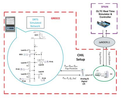
Figure 12. Test setup using JaNDER.
