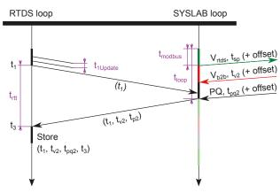
Figure 6. Time exchange protocol and associated loops.
