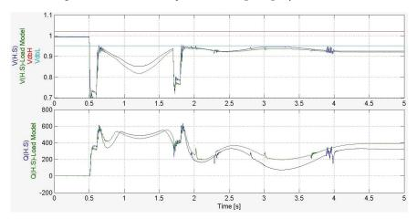
**Figure 12.** A 765 kV line fault nearby Shin-Jecheon bus considering induction motor and ZIP load model; Shin-Jecheon bus voltage (first row) and reactive power of SVC (second row); RTHS (blue line) and large-scale RTS (green line).
