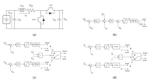
Figure 5. (a) Battery DC-DC circuit diagram. (b) DC voltage droop control, (c) DC voltage forming control, (d) battery current control.
