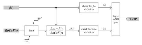
Figure 2. A simplified logical diagram of the innovative UFLS process.
