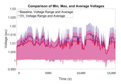
Figure 8. Volt-Var (VV) vs baseline feeder voltage comparison.
