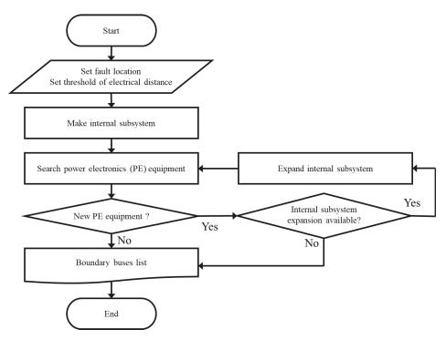
Figure 6. The procedure of determination of boundary buses.
