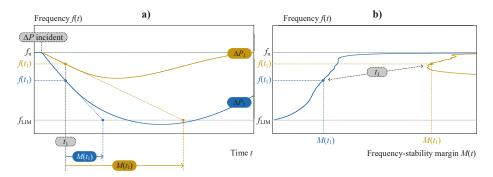
**Figure 1.** EPS frequency f(t) response to different  $\Delta P$  incidents (**a**) and the corresponding frequency versus frequency stability margin diagram (**b**).
