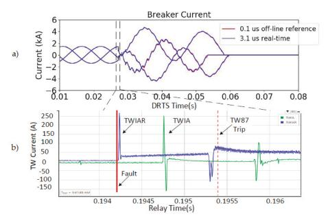
**Figure 8.** Results for testing a commercial travelling-wave relay for a three-phase to ground fault: simulation results for (**a**) three-phase current on the faulted line at the remote bus and (**b**) relay current variables.
