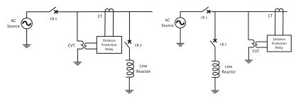
(a) Relay fed through CT connected before reactor. (b) Relay fed through CT connected after reactor Figure 4. Connection point of current transformers (CTs) for Case 1 (a) and 2 (b).
