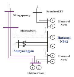
Figure 13. Single line diagram near TCSC.
