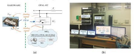
**Figure 11.** HIL setups [43]. Reproduced with permission from Hyeong-Jun Yoo, A Droop Frequency Control for Maintaining Different Frequency Qualities in a Stand-Alone Multimicrogrid System; published by IEEE, 2018. (a) I/O signals between DSP and OP5600 for the  $MG_1$ ; (b) HIL platform for proposed MMG system.
