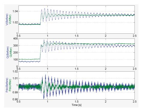
**Figure 3.** An example of parameter tuning experience during HILS-DPT; step-response test; voltage (first row), reactive power of STATCOM (second row), and active power of high-voltage direct current (HVDC; third row); before tuning (blue line) and after tuning (green line).
