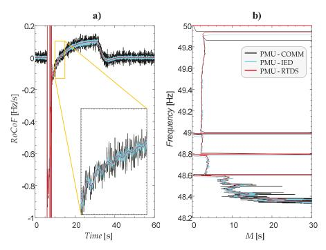
**Figure 5.** The *RoCoF(t)* report of three applied sources (PMU-IED, PMU-COMM and PMU-RTDS) after the RTDS simulation of an active power deficit and three UFLS interventions (**a**) and a corresponding frequency versus frequency stability margin diagram (**b**).
