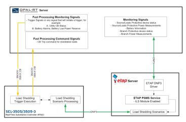
**Figure 16.** Generic microgrid controller CHIL testbed [41]. Reproduced with permission from Elsevier, A generic microgrid controller: Concept, testing, and insights; published by Elsevier, 2018.
