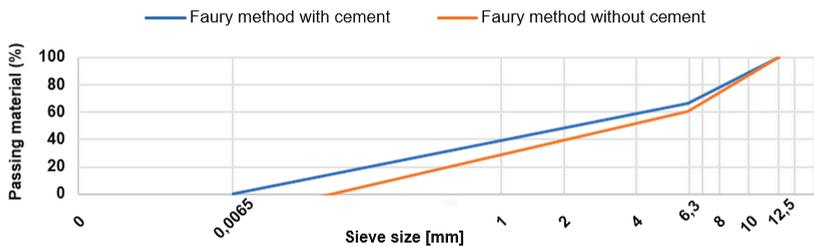
Figure 1. Faury method for reference concrete.
