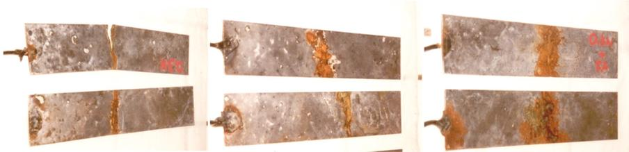
**Figure 7.** Visual observation of the corrosive attack on the bare steel plates in reference natural aggregate concrete (Nat-0.6, on the left), in recycled aggregate concrete (Rec-0.3, in the middle), and high-volume fly ash concrete (Nat + FA-0.6, on the right).
