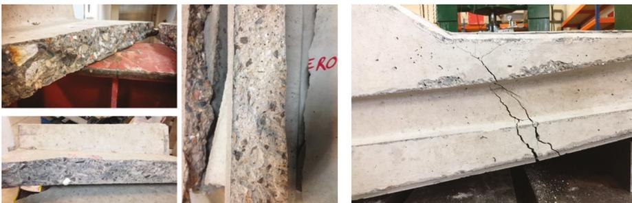
**Figure 11.** Precast test and cracking.
