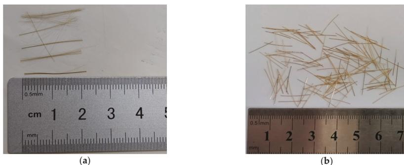
Figure 1. Fiber: (a) Basalt fiber (b) Steel fiber.
