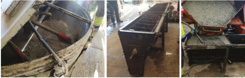
Figure 2. Precast element manufacturing sequence.
