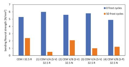
**Figure 10.** Bending flexural strength without and with frost impact evaluated after 90 days of water curing (each value as mean value of 3 individual tests).
