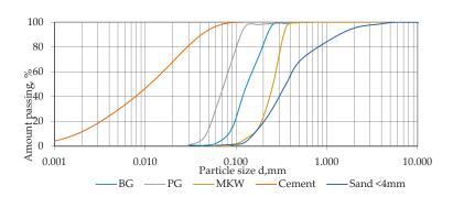
Figure 1. The particle size distribution of the raw materials used to prepare novel building material.
