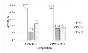
Figure 7. The porosity of alkali activated fine-grained concrete samples. P—total porosity; Pa—open porosity; Pu—closed porosity.
