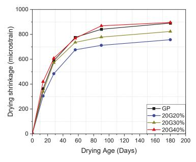
Figure 3. Drying shrinkage of SCC mixes containing glass powder with 20  $\mu m$  particle size at different replacement levels.
