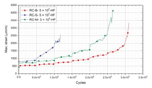
**Figure 9.** Maximum strain of high-frequency Locati fatigue tests with  $5 \times 10^5$  cycles per step.
