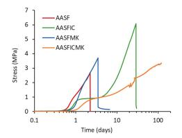
**Figure 4.** Autogenous-shrinkage-induced stress in AASF paste with SAPs and/or MK. A logarithmic scale is used on the x-axis in order to distinguish individual curves. The small fluctuation of the stress in AASFICMK paste on around 20 days and 30 days was due to the temperature fluctuation in the curing room.
