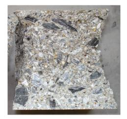
Figure 14. Concrete cube test specimen after compressive strength testing according to Table 7.
