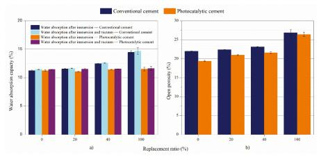
Figure 6. Comparison of results for (a) water absorption capacity and (b) open porosity.
