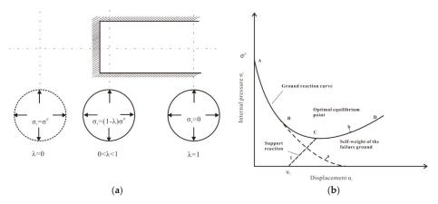
**Figure A1.** Convergence confinement method: (**a**) evolution of tunnel convergence with face advance; (**b**) ground reaction curve and support reaction curve (adapted from Orestes [13]).
