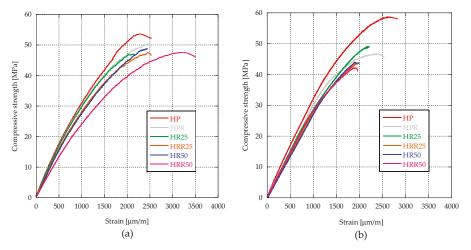
Figure 6. Compressive strength-strain at 160 (a) and 365 (b) days.
