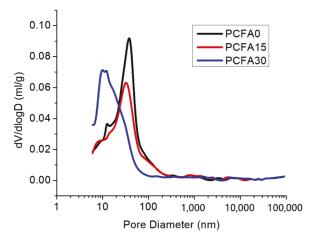
Figure 10. Pore size distribution after 90 days of curing.
