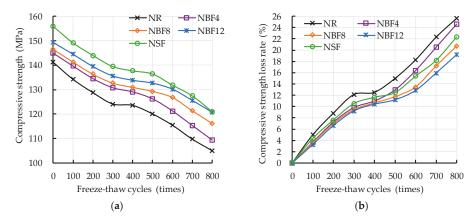
**Figure 7.** Compressive strength and compressive strength loss rate versus freeze–thaw cycles: (a) Compressive strength; (b) Compressive strength loss rate.
