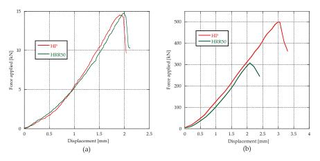
Figure 10. Mechanical characterization of precast elements: Bending test on ditches (a), impact test on barriers (b).
