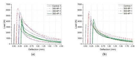
Figure 7. Bending test results of mixtures with 4 V%, 6 V% and 8 V% of (a) 300  $\mu$ m fibers and (b) 500  $\mu$ m fibers.
