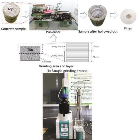
(c) Concentration titration of chloride ions.
