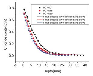
Figure 4. Regression curves of chloride coefficient using Fick's second law (by mass%).
