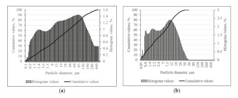
Figure 2. Granulometric composition of biomass bottom ash (a) and phosphogypsum (b). The mean diameter of PG particles is 74.7  $\mu$ m and for the particles of BBA is 58.6  $\mu$ m.
