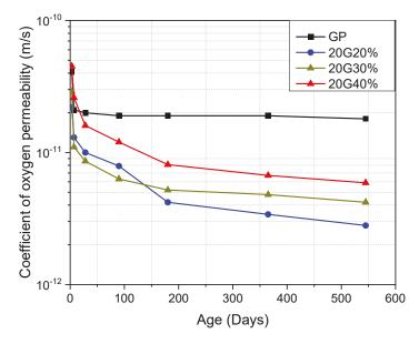
Figure 5. Coefficient of permeability of SCC mixes containing glass powder with 20  $\mu$ m particle size at different replacement levels.
