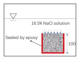
(a) Concrete sample immersion in NaCl solution.
