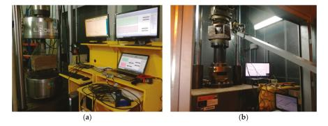
Figure 3. Fatigue tests. (a) Low-frequency fatigue testing and (b) high-frequency fatigue testing.
