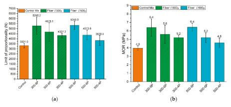
Figure 8. Bending test assessment: (a) limit of proportionality F<sub>max</sub>; (b) modulus of rupture.
