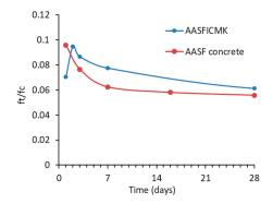
Figure 7. Splitting tensile strength-to-compressive strength  $(f_t/f_c)$  ratios of AASFICMK concrete, in comparison with AASF concrete.
