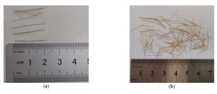
Figure 1. Fiber: (a) Basalt fiber (b) Steel fiber.
