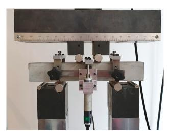
Figure 3. Four-point bending test performed according to ASTM C1609 [52].
