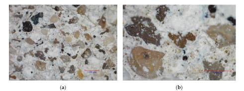
Figure 2. Macrostructure of ternary system mortar (a) under magnification of 40x, (b) under magnification of 120x.
