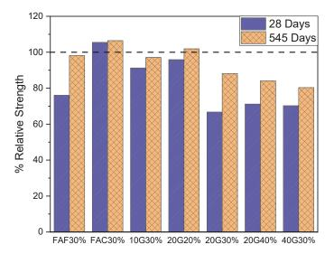
**Figure 1.** Relative strength of mixes normalized with respect to general purpose (GP) mix at the respective age.
