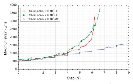
**Figure 10.** Comparison of the maximum strain of the RC-B for a Locati test with  $2 \times 10^5$  cycles per step at a low frequency (RC-B-MF-2 × 10<sup>5</sup>), a Locati test with  $2 \times 10^5$  cycles per step at a high frequency (RC-B-HF-2 × 10<sup>5</sup>) and a Locati test with  $5 \times 10^5$  cycles per step at a high frequency (RC-B-HF-5 × 10<sup>5</sup>).
