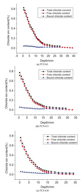
Figure 5. Distribution of total chloride, free chloride, and bound chloride in concrete samples (by mass%).
