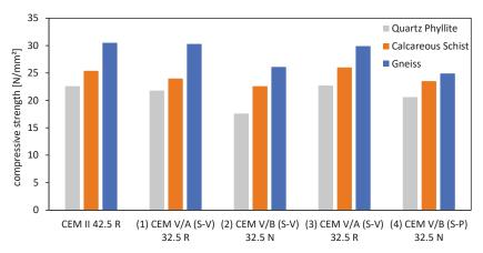
**Figure 13.** Compressive strength of various concrete mixtures varying cement and aggregate type (each value as mean value of 3 individual tests) after 28 days.
