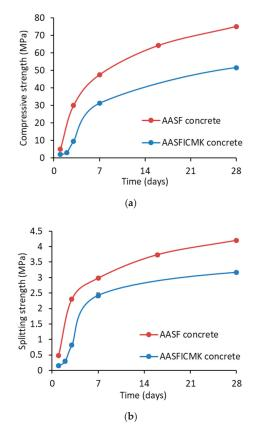
**Figure 6.** Compressive (**a**) and splitting strength (**b**) of AASFICMK concrete in comparison with AASF concrete. For splitting strength, the error bar is shown in the diagram, but it is too small to be clearly distinguished from the marker.
