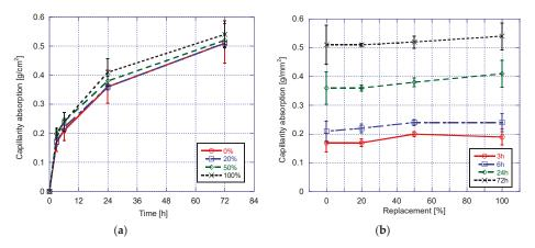
Figure 3. Capillarity absorption vs. time (a) and capillarity absorption vs. replacement ratio (b).
