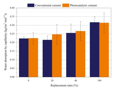
Figure 5. Water absorption by capillarity comparison.
