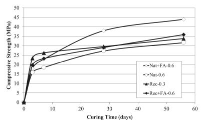
Figure 2. Compressive strength vs. curing time.
