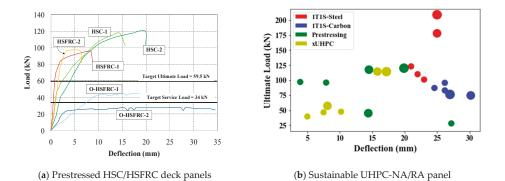
Figure 7. Load deflection responses of prestressed deck panels.
