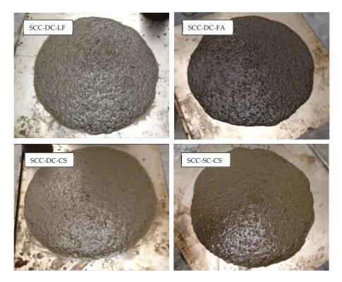
Figure 2. Slump disks detail of all mixes.
