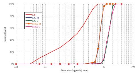
Figure 1. Grading of the aggregates.
