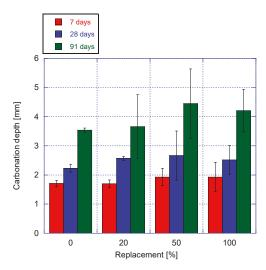
Figure 9. Carbonation depth for all mixes and ages.
