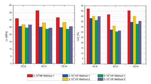
**Figure 13.** Comparison of the high-frequency fatigue limit obtained using five different procedures and the low-frequency fatigue limit.
