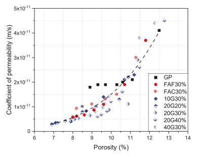
Figure 9. Relationship between coefficient of permeability and porosity.
