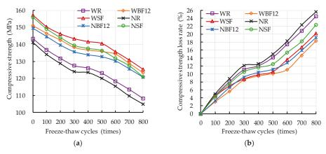
**Figure 9.** Compressive strength and Compressive strength loss rate versus freeze–thaw cycles: (a) Compressive strength; (b) Compressive strength loss rate.
