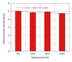
Figure 8. Ultrasonic pulse velocity at 28 days.
