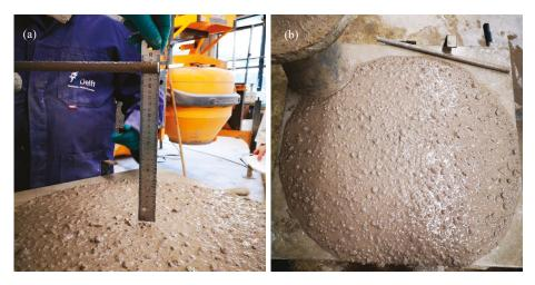
Figure 5. Slump (a) and flowability (b) of AASFICMK concrete.
