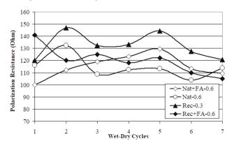
Figure 6. Polarization resistance of bare steel plates in cracked concrete as a function of wet-dry cycles.
