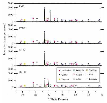
Figure 4. X-ray diffraction patterns of photocatalytic mortar family.
