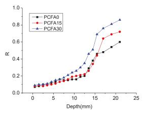
Figure 8. Relation between chloride bound capacity amount and concrete depth.
