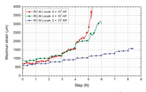
**Figure 12.** Comparison of the maximum strain of the RC-M for a Locati test with  $2 \times 10^5$  cycles per step at a low frequency (RC-M-MF- $2 \times 10^5$ ), a Locati test with  $2 \times 10^5$  cycles per step at a high frequency (RC-M-HF- $2 \times 10^5$ ) and a Locati test with  $5 \times 10^5$  cycles per step at a high frequency (RC-M-HF- $5 \times 10^5$ ).
