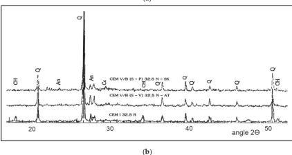
**Figure 3.** XRD diagrams displaying angle 2 $\Theta$ -intensities of (**a**) CEM V/A types and reference cement CEM I and (**b**) CEM V/B types and reference cement CEM Iafter 365 days curing at 20 °C under water, whereby: CH—portlandite Ca(OH)<sub>2</sub>; Cc—calcite, Q—quartz SiO<sub>2</sub>, An—anorthite (CaAl<sub>2</sub>Si<sub>2</sub>O<sub>8</sub>).
