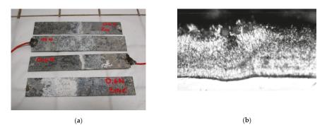
Figure 10. Visual obs. (a) and metallographic cross section (b) of galvanized steel plate in Nat-0.6
