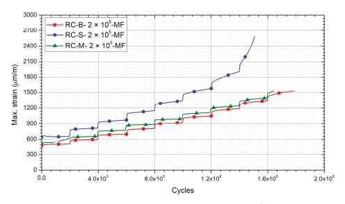
Figure 6. Maximum strain of low-frequency Locati fatigue tests with  $2 \times 10^5$  cycles per step.
