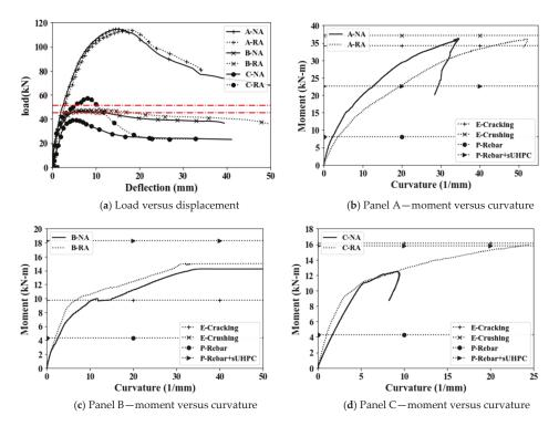
Figure 9. Load deflection responses of composite deck panels.
