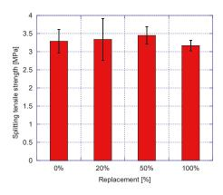
Figure 5. Tensile strength of all mixes at 28 days.
