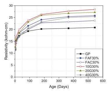
Figure 10. Electrical resistivity of SCC mixes at 30% cement replacement at different ages.
