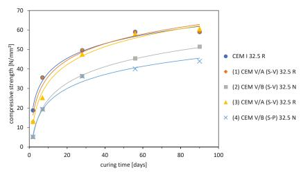
Figure 4. Compressive strength development of standard mortar specimens according to [51] (each value as a mean value of 3 individual tests), after 2, 7, 28, 56, and 90 days.
