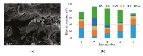
**Figure 5.** Energy Dispersive Spectroscopy (EDX) analysis of GCP-PG binder. (a) point positions analyzed by EDX, (b) element content in analyzed region.
