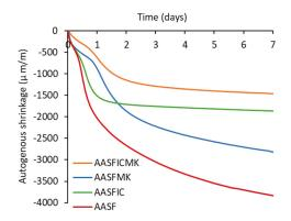
Figure 3. Autogenous shrinkage of AASF paste with SAPs and/or MK.
