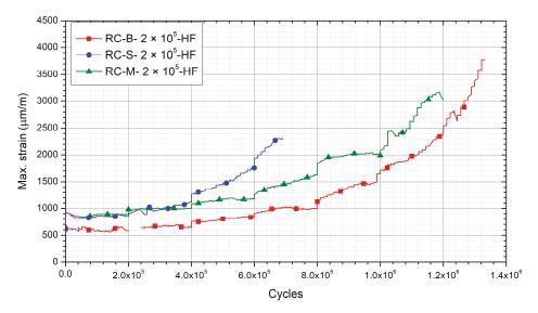
**Figure 7.** Maximum strain of high-frequency Locati fatigue tests with  $2 \times 10^5$  cycles per step.
