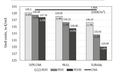
Figure 2. Cost of shotcrete for each composition, assuming different cost scenarios of the recycled aggregates.
