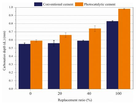
Figure 8. Carbonation depth comparison at 56 days.
