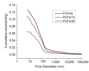
Figure 9. Cumulative porosity of concrete sample with different fly ash additions after 90 days of curing.
