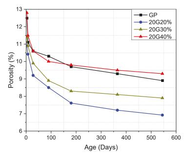
Figure 8. Porosity of SCC mixes containing glass powder with 20  $\mu$ m particle size at different replacement levels.
