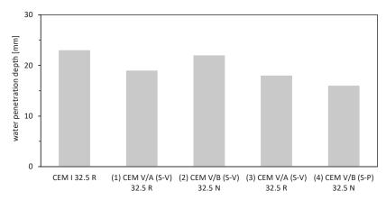
**Figure 12.** Water penetration depth (in mm) after water pressure test (each value as mean value of 3 individual tests).
