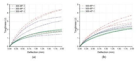
**Figure 9.** Cumulative toughness of the bamboo fiber reinforced specimens up to 2 mm deflection: (**a**) 300  $\mu$ m batch; (**b**) 500  $\mu$ m batch evaluated from the four-point bending test according to ASTM C1609 [52].
