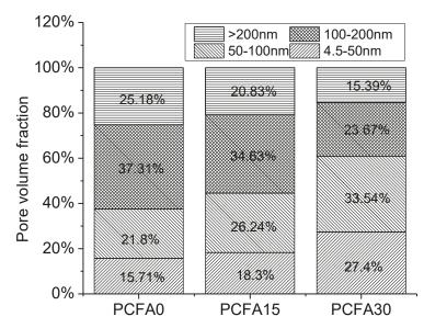
Figure 11. Pore size distribution of concrete with different fly ash additions after 90 days of curing.
