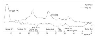
**Figure 1.** XRD diagrams displaying angle 2 $\Theta$ -intensities of cementitious constituents fly ash (V) and furnace slag (S), whereby: Alite—3CaO × SiO<sub>2</sub>; Belite—2CaO × SiO<sub>2</sub>; Celite—2CaO × Al<sub>2</sub>O<sub>3</sub>; Ferrite—4CaO × Al<sub>2</sub>O<sub>3</sub> × Fe<sub>2</sub>O<sub>3</sub>.
