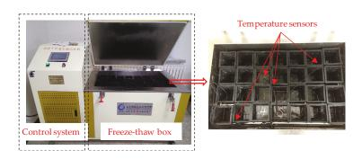
Figure 3. Freeze-thaw cycle test.
