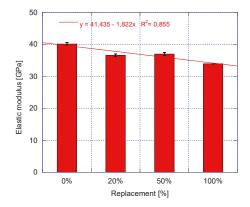
Figure 7. Modulus of elasticity of all mixes at 28 days.
