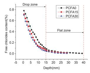
Figure 2. Free chloride deposition of concrete with different fly ash replacement ratios.
