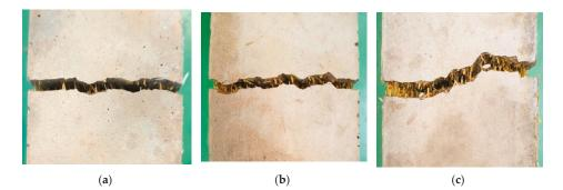
**Figure 6.** Photographs of test samples after bending tests involving 500  $\mu$ m fibers. Fiber content: (a) 4 V%, (b) 6 V% and (c) 8 V%.
