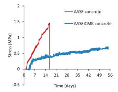
Figure 9. Self-induced stress in AASF and AASFICMK concrete.
