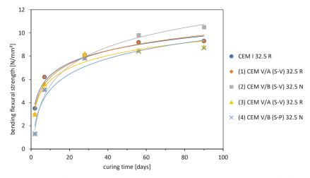
Figure 5. Bending flexural strength development of standard mortar prisms according to [51] (each value as mean value of 3 individual tests), after 2, 7, 28, 56, and 90 days.
