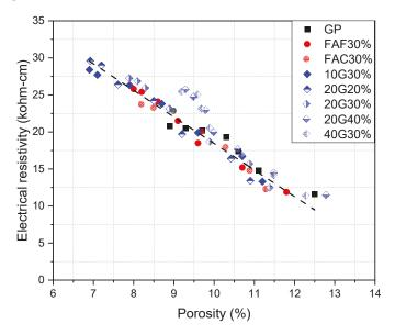
Figure 12. Relation between electrical resistivity and porosity.
