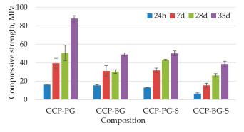
Figure 6. The compressive strength of ternary binder and mortar.
