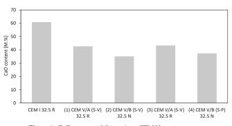
Figure 2. CaO content of the various CEM V cement types.
