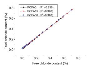
Figure 7. Relation between free chloride and total chloride depth (by mass%).
