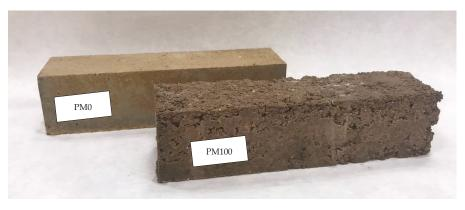
Figure 1. Porous appearance of PM100 versus smooth appearance of other mixes.
