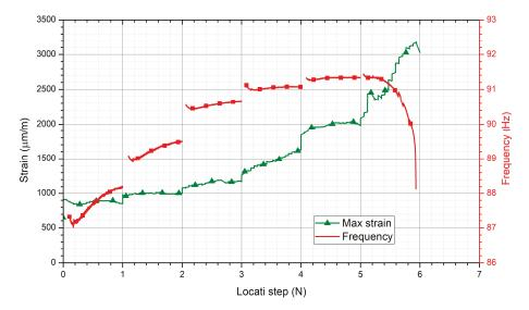
**Figure 8.** Maximum strain and resonance frequency comparison during high-frequency Locati fatigue tests with  $2 \times 10^5$  cycles per step.
