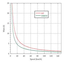
Figure 12. Simulated behavior of reinforced barriers.
