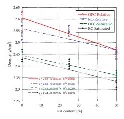
Figure 4. Density vs. RA content.
