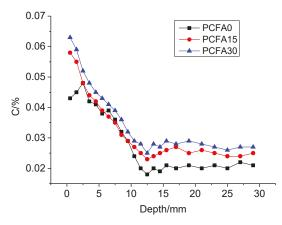
Figure 6. Relationship between bound chloride amount and concrete depth (by mass%).
