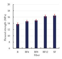
Figure 5. Effect of basalt fiber content and fiber type on the flexural strength of RPC.
