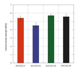
Figure 9. Tensile splitting strength at 90 days for all mixes.
