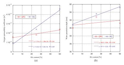
Figure 8. Oxygen permeability coefficient (a) and water penetration depth (b).
