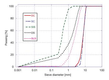
Figure 1. Aggregates granulometric grading.
