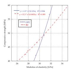
Figure 7. Compressive strength vs. modulus of elasticity.
