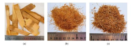
**Figure 1.** Bamboo fibers. (a) Raw waste material; (b) 300 µm-diameter fibers after grinding and sieving; and (c) 500 µm-diameter fibers after grinding and sieving.
