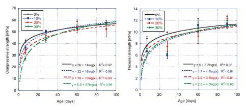
Figure 4. Mechanical properties of mortars with several cement replacements with cupola slag.
