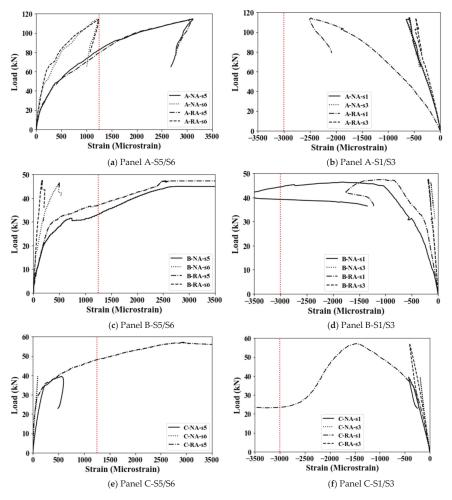
Figure 11. Load-strain responses for the composite deck panels.
