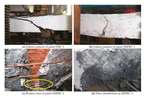
Figure 8. Failure pattern and forensics of prestressed panels.
