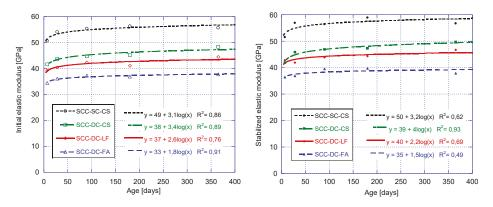
Figure 8. Evolution of the initial elastic modulus (left) and the stabilized elastic modulus (right) for the different concrete mixes.
