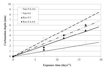
Figure 3. Carbonation depth vs. time of air exposure.
