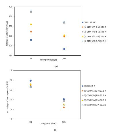
Figure 6. Development of total porosity (a) and percentage of macro-porosity (b) for a curing time of 28 and 365 days.
