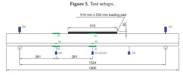
Figure 6. Instrumentation plan.
