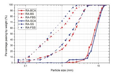
Figure 1. Aggregate grading curves.
