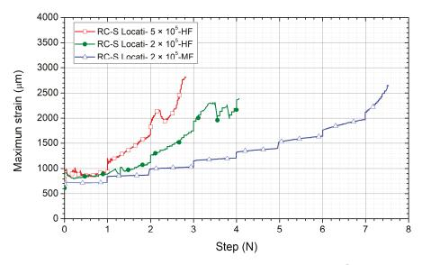
**Figure 11.** Comparison of the maximum strain of the RC-S for a Locati test with  $2 \times 10^5$  cycles per step at a low frequency (RC-S-MF- $2 \times 10^5$ ), a Locati test with  $2 \times 10^5$  cycles per step at a high frequency (RC-S-HF- $2 \times 10^5$ ) and a Locati test with  $5 \times 10^5$  cycles per step at high frequency (RC-S-HF- $5 \times 10^5$ ).
