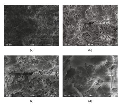
**Figure 3.** Microstructure of the ternary binder detected by SEM in magnification of 500x and 1000x. (**a**,**c**) GCP-phosphogypsum (PG), (**b**,**d**) GCP-BG.
