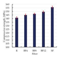
Figure 4. Effect of basalt fiber content and fiber type on the compressive strength of RPC.
