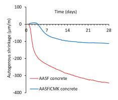
Figure 8. Autogenous shrinkage of AASF and AASFICMK concrete.
