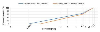
Figure 1. Faury method for reference concrete.
