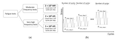
Figure 2. (a) Experimental fatigue campaign. (b) Locati methodology description. MF: moderate frequency, HF: high frequency.
