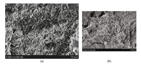
Figure 6. Microstructure of alkali activated biomass bottom ash samples (a) PG 15-3 and (b) PGWG 15-3.
