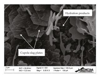
Figure 6. Appearance of the cupola slag after reacting on the cement paste (5000×).
