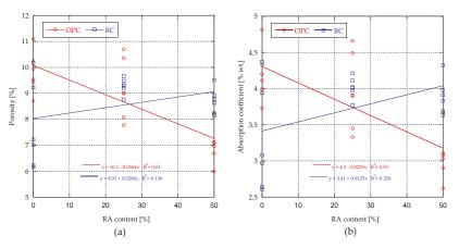
Figure 5. Porosity (a) and absorption coefficient (b) vs. RA content.
