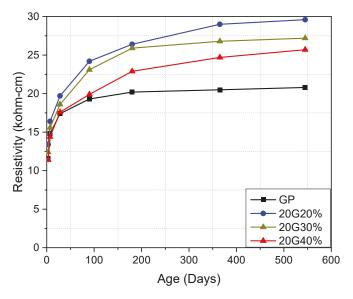
Figure 11. Electrical resistivity of SCC mixes containing glass powder with 20  $\mu$ m particle size at different replacement levels.
