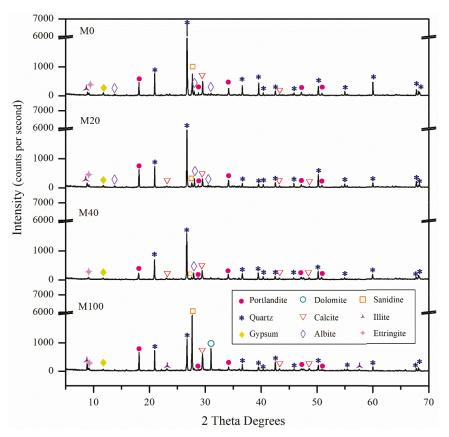
Figure 3. X-ray diffraction patterns of conventional mortar family.
