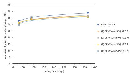
**Figure 9.** Modulus of elasticity (static) using different cement types at 2, 28, and 90 days of water curing (each value as mean value of 3 individual tests).
