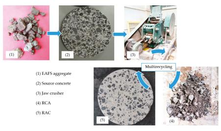
Figure 2. Recycled aggregate concrete (RAC) manufacturing process.
