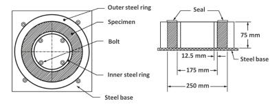
Figure 1. Dimensions of the steel rings, after [22].
