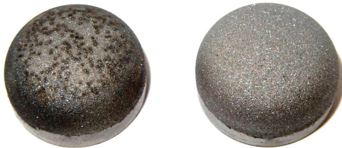
Figure 3. Plug-type contact with diameter 19 and 10 mm length in new (right) and worn condition after test (left). The surface has a biradial shape with a radius of 5 mm at the side and 20 mm at the tip, respectively.
