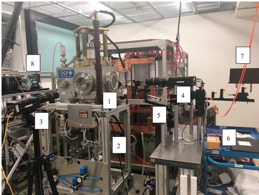
Figure 1. Setup for studies on vacuum arcs: (1) vacuum chamber, (2) pumping system, (3) high-speed camera (general arc dynamics), (4) two high-speed cameras equipped with narrow-band optical filters, (5) NIR optics, (6) NIR spectrometer, (7) Xe flash lamp, (8) 0.75 m imaging spectrograph.
