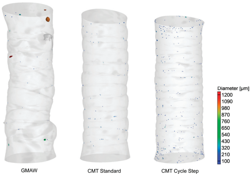
Figure 11. Computer tomography scans with porosity analysis of the conventional GMAW bar, the CMT standard bar, and the CMT cycle step bar.
