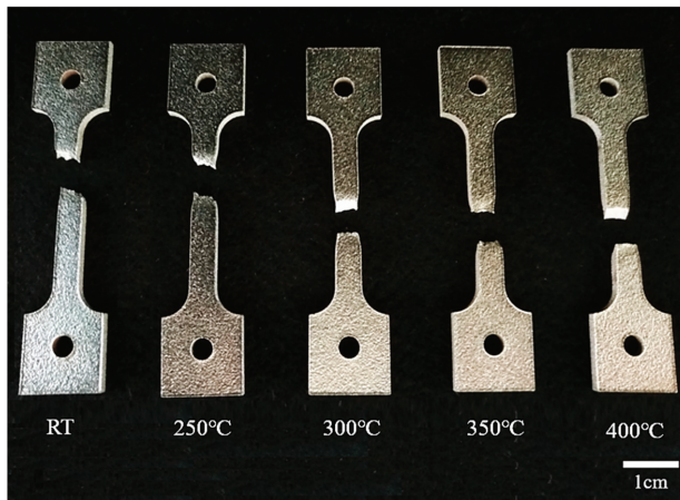
Figure 10. Macroscopic morphology photographs of room temperature and high temperature tensile fracture specimens.
