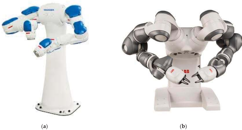
Figure 6. Robotic structure with two robotic arms: (a) Yaskawa type [12]; (b) ABB type [13].
