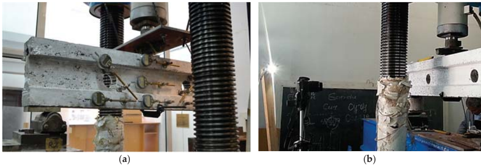
Figure 3. Equipment for beams. (a) The set-up of the mechanical gauges and displacement transducer. (b) The equipment required to apply the optical method (DIC).
