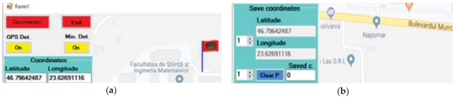
Figure 10. User-adapted graphic interface and the communication tool between the client and server: (a) coordinates definition; (b) data saving tool in the user interface and map location monitoring.
