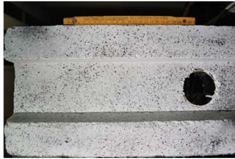
Figure 4. Speckle pattern on the surface of the analyzed area.
