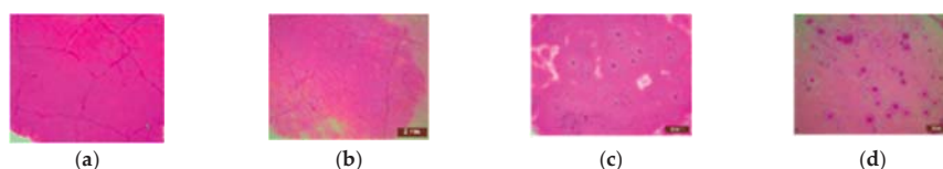
Figure 6. Discoloration of test specimens following the test diagram, example P1—control specimen made of the cementitious composite without TiO 2 content: before (a) and after (b) the test diagram, with luminous intensity 860 lux; before (c) and after (d) the test diagram, with luminous intensity 405 lux.
