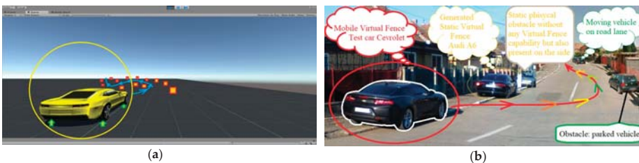
Figure 7. The Chevrolet Camaro was equipped with MVF both in the digital and actual drive test environment: (a) Robotic virtual modeled vehicle using the self-driving optimization capacity to avoid objects; (b) driver assistance system was applied to validate the virtual distilled model of the robotic car.
