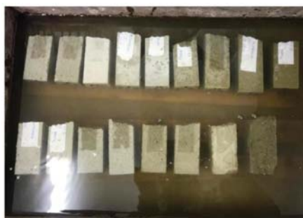
Figure 2. Fully water-soaked specimens.
