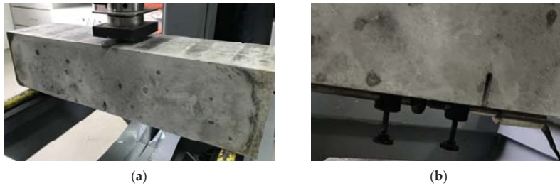
Figure 2. Flexural tensile strength: (a) loading scheme of the samples; (b) transducer used for the displacement measurement.
