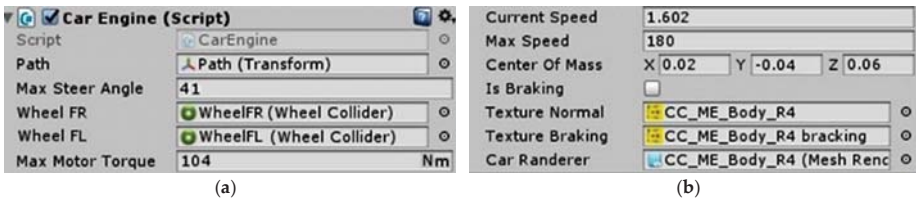
Figure 5. Basic digital support in configuring the car control program script in Unity 5 application: (a) Car engine script used to define maximum motor torque; (b) kinematic parameter definition.
