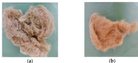
Figure 4. Retama monosperma stem fibers. (a) Before manual carding; (b) after manual carding.
