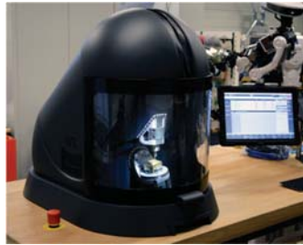
Figure 1. The Micro5, the milling machine used in this study.
