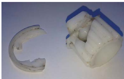
Figure 1. Broken grooved shaft–plastic material/part.
