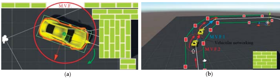
Figure 4. Robotic Chevrolet Camaro model supported by mobile virtual fence (MVF) in the Unity 5 virtual reality drive test: (a) Digital model of tested robotic vehicle is self-driving away from an obstacle; (b) vehicular mobile networking when both cars communicate and interact through their MVFs.
