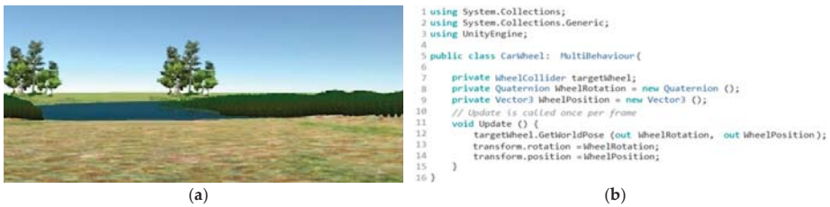
Figure 2. Basic programming results in virtual reality program Unity 5: (a) Environment used for track generation for digital testing of the robotic car; (b) sequence of the program used for automation of the Chevrolet Camaro robotic model.
