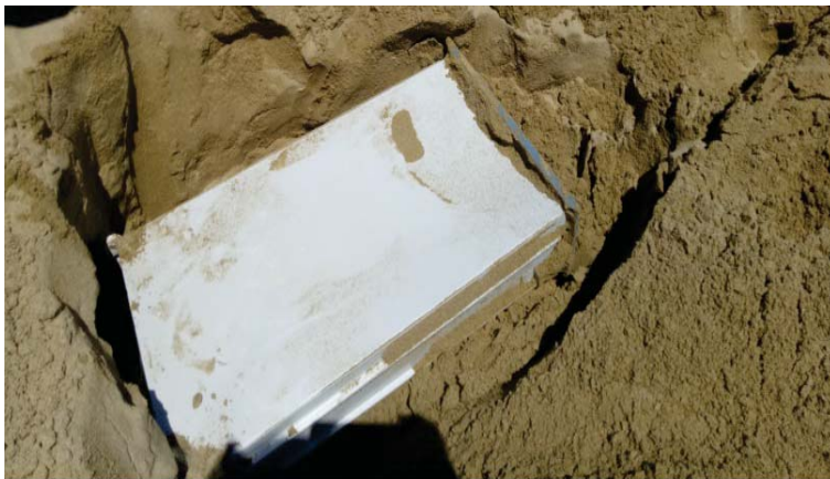
Figure 6. Image of a conductive object with dimensions 0.61 \times 0.35 m.
