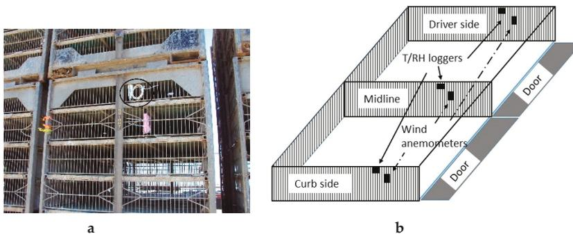
**Figure 3.** (a) Thermal and wind dataloggers secured on curbside of a transport module during a monitoring campaign. (b) Diagram of instrumented transport drawers showing loggers on curbside, midline and driver side. The interior loggers consist of those on the midline, while exterior loggers consist of those on driver and curbsides.
