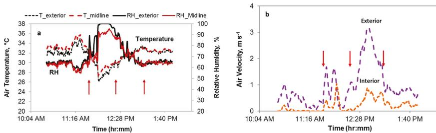
**Figure 5.** Temperature, relative humidity (a) and air velocity (b) profiles from interior and exterior logger positions of a summer trip. The first arrow on each graph indicates the beginning of loading, the second the beginning of transport, and the third the beginning of holding period.
