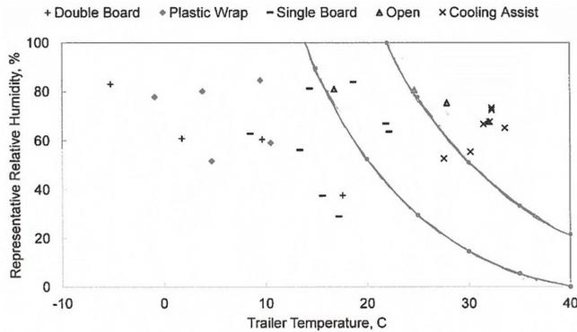
**Figure 6.** Average representative relative humidity vs. average trailer temperature of 28 monitored trips moving broilers to processing plants. The AET values corresponding to 40 and 65 °C [17] were overlaid.
