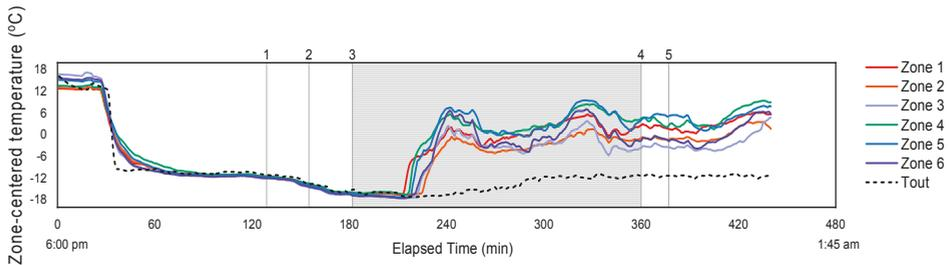
**Figure 5.** Ceiling-centered temperature profile representing 6 zones inside a pig trailer during a *Very Cold* evening trip. Zones 1 to 3 representing trailer top deck, and Zones 4 to 6 representing bottom deck. Events occurred during the trip are numbered on the figure as follows: 1. Arrival at a commercial pig barn; 2. Loading; 3. En route; 4. Arrival at abattoir; 5. Unloading.
