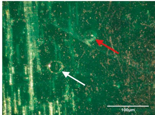
**Figure 1.** Light micrograph of uninoculated fiberglass flooring material depicting a hole (white arrow) in the material as well as subsurface air bubbles (red arrow). Sub-surface bubbles can be exposed to surface contamination as the surface wears with age.
