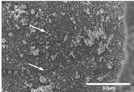
**Figure 4.** Micrograph of the bottom of the hole seen in Figure 3. Large aggregates of bacteria are evident adhering to the area of the hole (white arrows). Figures 2–4: Scanning electron micrographs of bacteria inoculated flooring at various timepoints after inoculation and magnifications.
