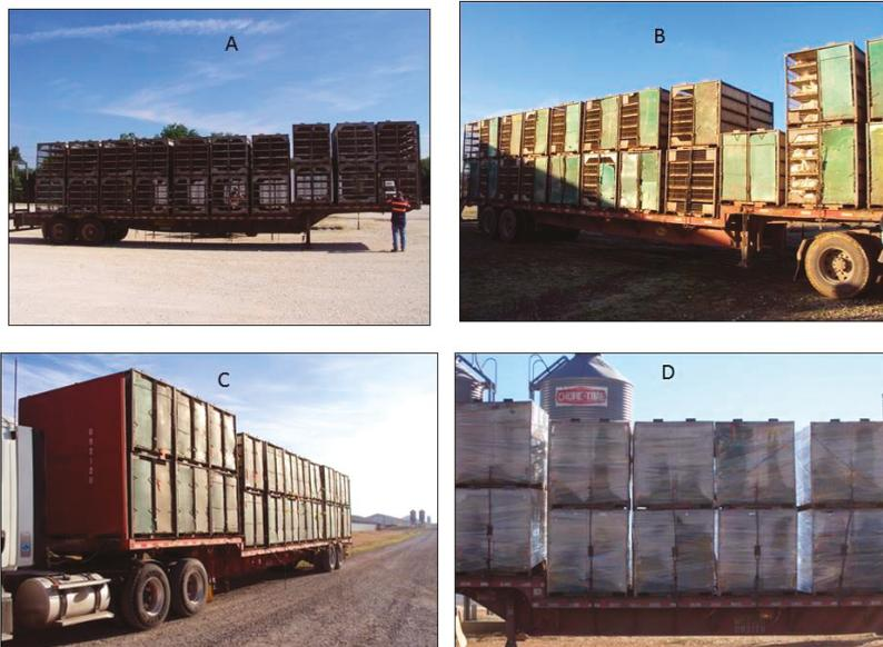
**Figure 2.** Weather-dependent trailer configurations employed by companies. **A.** Open, used for hot and mild seasons; **B.** Single board, used when transitioning between mild and winter seasons; **C.** Double board used in winter seasons; **D.** Plastic wrap on double board modules, used in winter days or nights with extremely cold conditions.
