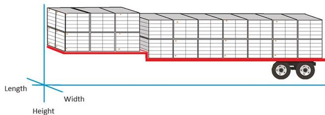
**Figure 4.** Schematic of an industry-standard drop deck poultry trailer loaded with 20, 10-door modules. Dataloggers (shown as orange dots) for temperature were installed as a  $5 \times 3 \times 3$  grid on the trailer. Three horizontal planes along height are Top, Middle, and Bottom. Three longitudinal planes along width are Driver, Midline and Curb.
