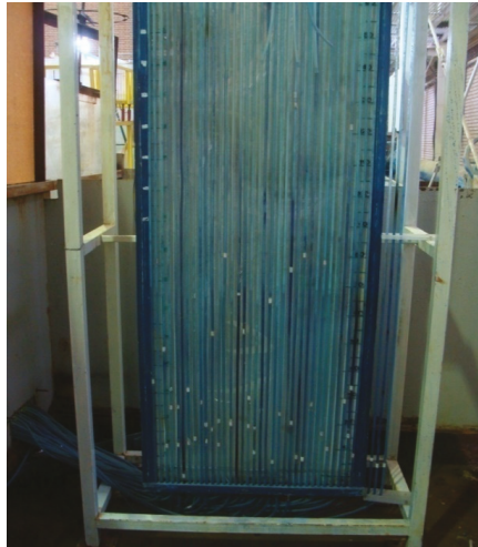
Figure 3. The 37 piezometers connected to impact plate for observation of dynamic pressure fluctuations.
