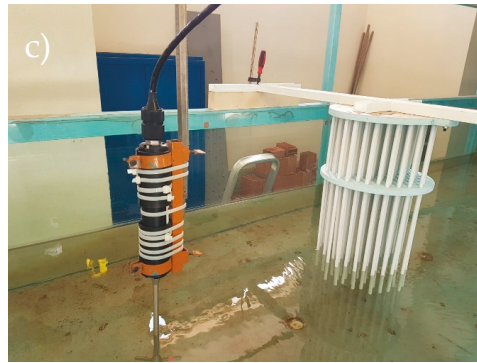
Figure 4. Photos from vegetation patches for different SVFs (Solid Volume Fractions): (a) side view, (b) top view, (c) view from an experiment with an Acoustic Doppler Velocimeter (ADV).
