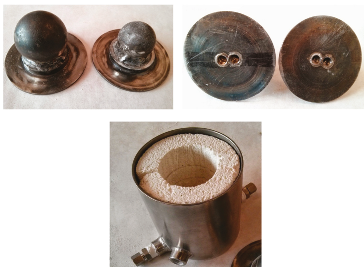
Figure 3. Scheme of the device for cooling molten material with metal spheres and views of the containment vessel.
