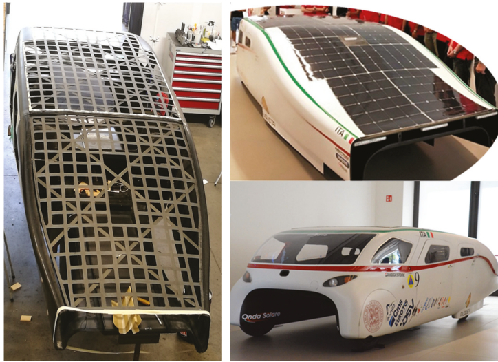
Figure 8. Solar roof manufacturing and installation on the solar vehicle.
