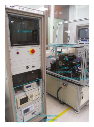
Figure 7. Experimental setup.
