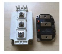
**Figure 5.** The 1.2 kV SiC MOSFET power module, part no. CAS120M12BM2, used in the project, with a rated current of 138 A (left) and a 36% smaller 1.2 kV SiC MOSFET power module, part no. CAB450M12XM3, with a rated current of 409A, available on the market from mid-2019.
