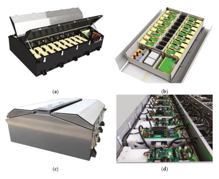
**Figure 4.** Assembly of power electronic cells of the DC PETT on the roof surface: (**a**) overall view of the whole device from the CAD program; detailed view of the 4QC-DAB-DC/AC power electronic cells and the LCL filter in the middle at the bottom (**b**); photos of the prototype (**c**) and (**d**).
