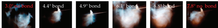
Figure A1. Comparison of the process glare for 1 mm and 1.5 mm flyer thickness at different collision angles, recorded by longtime exposure.
