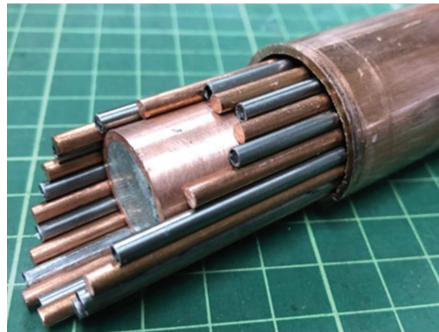
Figure 3. The pipe assembly of Sample B before explosive compaction (concentric outer and center copper pipe, inner solid copper bars, and steel pipes with paraffin).
