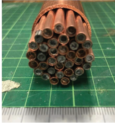
Figure 2. The pipe assembly of Sample A before explosive compaction (outer copper pipe, inner copper and steel pipes with paraffin).
